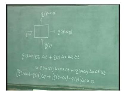
So we can write this as, q into x plus delta x minus qx into delta y plus qy plus delta y minus qy into delta x equal to 0. I just rearrange the terms and I can write that and from this, so I can write this the from here I can write this as qx plus delta x minus qy dividing the whole thing by delta x into delta y I can write this as qx plus delta x minus qx divided by delta x plus qy plus delta y minus qy divided by delta y equal to 0.
