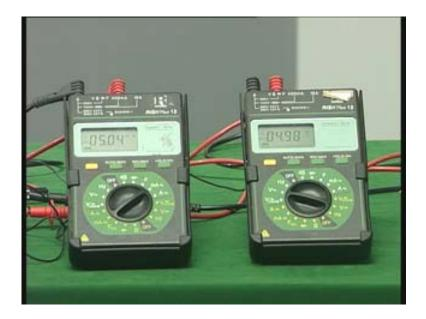
The input current is nearly more than 25mA. The rest of the 20mA will be flowing through the zener diode. Only 5mA flows through the load. The rest of the current is flowing through the zener diode.
