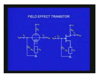
The circuit on the left is basically making use of a vacuum tube triode of the olden days. You have the coupling capacitors, you have the bleeding resistors  $R_{gl}$  as it is called and you have the cathode bias.  $R_k$  and  $C_k$  form the cathode bias for providing a bias for the triode and you have the  $R_p$  load resistor. This is a simple amplifier configuration using
