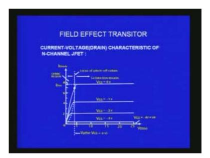
The current is going to be constant and dependent only on the voltage you applied between the drain and the source as well as the gate and source. I want to show very interesting thing with reference to the amplifier configuration. Here I have shown two circuits.
