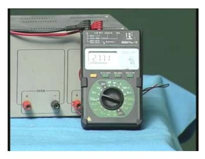
Now I will remove the voltmeter from across 270. I will connect it across 220. So I connect the positive to one end; I connect the negative to the other end. Now let us see what is the voltage? The previous one was 2.77, now it is 2.24.
