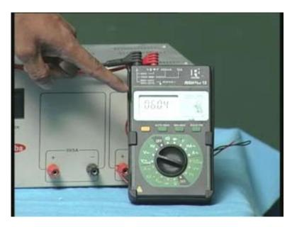
What I have applied is 6V. I have measured that. This is the voltage source. Now what I am going to do is I am going to measure the voltage across each of the resistors. So let me connect to one end of the resistor the negative terminal of the multimeter, to the other end I connect the positive terminal. So now I have connected the voltmeter across the 270 ohms here and voltage is around 2.77. I hope you can see that. The voltage here is 2.77 voltage.
