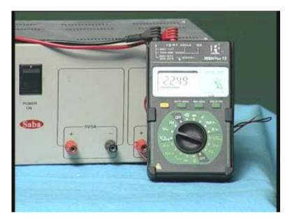
So if you add them together they come to approximately about 5V and now the last resistor is  $R_3$ , 100 ohms. I will connect the voltmeter across this 100 ohms here and at the bottom and you can see the voltage is about 1V.
