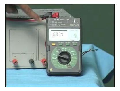
So totally 2.77+2.24+1 together gives me 6V approximately. So you can see whatever voltage I connected here is divided across each of these resistors. As Kirchoff's law says the voltage source should be equal to  $I_1R_1+I_2R_2+I_3R_3$  and therefore Kirchoff's law is verified.
