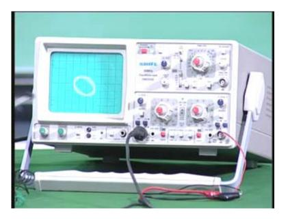
That shows the two frequencies are equal. Now if I make it into a dual slope both the sine waves are almost coinciding and the frequency is the same.
