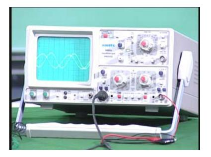
It is around 636. That is what you see here. This is the frequency and if you actually calculate 1 by 2 pi RC with R 1 kilo ohm and C 0.1 you will get close to 600 hertz but you may not get exact value and that is because there is also a tolerance of these resistors and the capacitors. Because of that you will not get an exact value but you should get very close value corresponding to 600 hertz.
