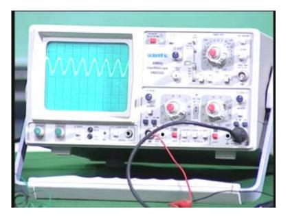
This is 10K the two resistors and the capacitors are 0.1 microfarad and this will be 2C. That means 2 times 0.1; 0.2 micro farad. Actually parallel capacitors are put there to add and this is 5K. They have put again resistors in parallel to make these 5K or you can use 4.7K. A very simple sinusoidal oscillator can be constructed using Twin-T network.
