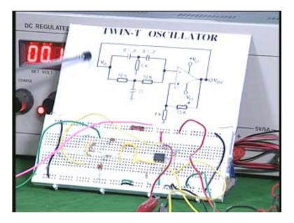
You can see the one T here one T here. The corresponding circuit is shown with two resistors and one capacitor and the two resistors and one capacitor here. This is the Twin-T network and you have the operational amplifier and one of the resistors here is made as a variable resistor for adjusting the gain and you observe in the oscilloscope the sine wave generated due to the twin-twin network.
