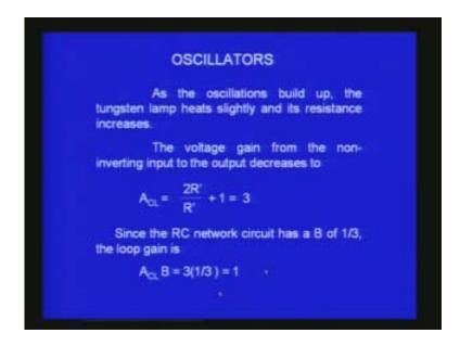
The closed loop gain is 2R prime by R prime plus 1 which is equal to 3 in this case and beta is 1 by 3. 3 into 1 by 3 is 1. That corresponds to Barkhausen's condition.
