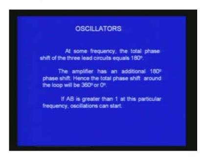
At some definite frequency f, 2 pi f will be omega and that will introduce at that frequency exact 180 degree phase difference with the combination of three RC networks. Once that happens you get the oscillations and when the AB is just the right value equal to 1 corresponding to Barkhausen condition the oscillations will start and you will get the
