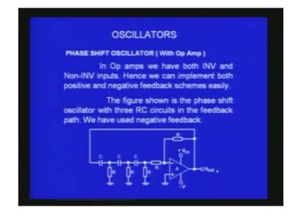
This is the circuit corresponding to a phase shift oscillator using op amp. You didn't find much difference with the transistor amplifier except that I have removed the transistor common emitter amplifier and in place of that I have introduced an inverting amplifier using op amp.
