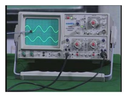
I have clamped it positive. I will show you again and again, number of times so that you can see on the screen that initially it is symmetric. When I dc couple it the whole sinusoidal wave moves up. That means it is positively clamped. That is what we see here.
