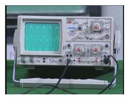
This is a positive clipper and if I want a negative clipper all that I have to do is change the direction of diode and change the reference voltage on this side. Then you will be able to get the negative clipping and you can also do a square wave clipping. That is both sides clipping, dual clipper both positive and negative by using Zener diode or combination of such circuits.
