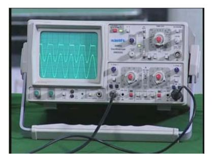
You can see the bottom one is the input signal, the top one is the clipped signal. You can see the clipping there. The clipping can be modified by changing the wiper position or by changing the reference voltage here. That is done by changing the potentiometer here. When I change the potentiometer I am able to change the point at which the signal is clipped by moving the wiper. The reference voltage is what is being changed now and thereby I am able to change the clipping voltage.
