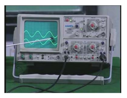
For the top one when I make it into dc still the sine wave is there and it has moved up to this line, the central line. It is symmetric to the central line and when I dc couple it, it moves up to this. That means the entire output has moved with reference to this as the reference line or zero line.
