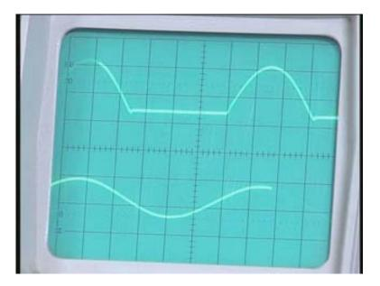
I will show you the next circuit which is a full wave rectifier signal. I want you to observe the circuit here. It is the same as what I discussed. The first circuit is an ideal half wave rectifier, precision half wave rectifier which we have already seen using an op amp and a diode and the second circuit is actually a summing amplifier with one input coming from here, the other input coming from the input.
