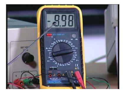
I again go back you will find again it comes to  $+V_{cc}$ . I go back again you wound find it becomes  $-V_{cc}$ . It is at this threshold that this happens and if you measure this it will be very close to 1.2 volts, the input at the positive input. That is at the non-inverting terminal. This shows that the comparator is capable of detecting voltages within the range of 1.2 volts, plus or minus 120 microvolt on either side and it can be used to compare two different voltages.
