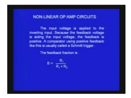
Some of you might have studied in transistor circuits that by using two transistors one can make a Schmitt trigger which is designed by the Schmitt as the name goes. What the circuit does is it is sensitive to some threshold voltage at the input and the output will go
