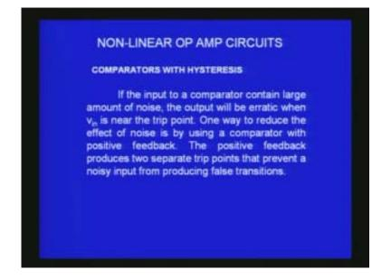
But this plus or minus 150 microvolt is what is called hysteresis for a reason which I will explain to you in a moment. It would be better in many applications to have this difference +150, -150 much larger than the small value. For example plus or minus 1 volts or plus or minus 2 volts as the case may be. This is because in every circuit there is always the noise component which are all unwanted signals coming from various sources all around us and some of them are harmonic.
