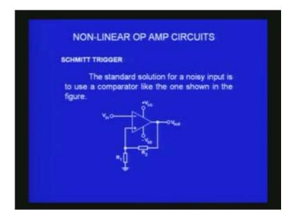
From plus or minus 150 microvolts we have now expanded the variation to plus or minus 1.2 volt which is a very large difference and this 1.2 volts cannot be generated by any of the noise voltage in normal course and we don't have to worry that the output is switching state because of the input noise. This is also called by another name Schmitt trigger.
