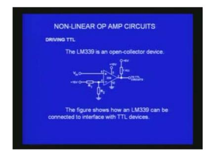
Because it is connected through an open collector output to 5 volts the output will be clamped at 5 volts and zero volts and it becomes compatible to TTL devices or digital circuits.
