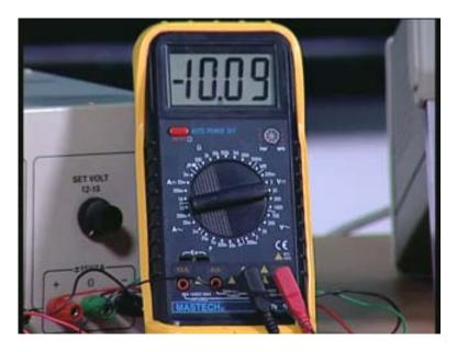
I can also do in another way. Now I bring back to 1 volt and vary this continuously. There is another dial here which can vary continuously. Now I would like you to watch the multimeter. As I keep increasing it you find when I just move by very small extent it has come to  $-V_{cc}$ .
