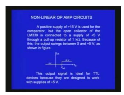
The pull-up resistor is around 1 kilo ohms. The transfer current for that circuit will be zero volts till I come to the  $V_{ref}$  and beyond that will be +5 volts. All these comparators so far that I talked about will have transition occurring at plus or minus 150 microvolts.
