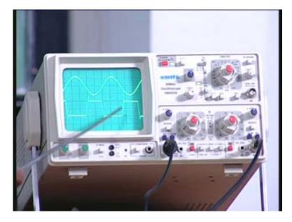
The input is sine wave and when I vary the amplitude you see the sine wave amplitude is also varying on the oscilloscope and what I get is a square wave at the output. This is the output.
