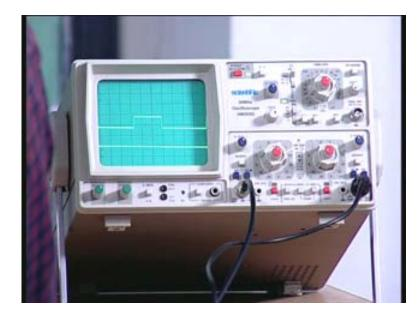
When I vary this nearly by half a scale it is changing. What we saw is a demonstration of the regenerative comparator where the input was given as a sine wave and the output is given as a positive feedback by having a resistor network  $R_1$  and  $R_2$  and when we change one of the potentiometers the output was also changing. That means the reference point was changing and it will have some effect on the output period or the frequency of the square wave.
