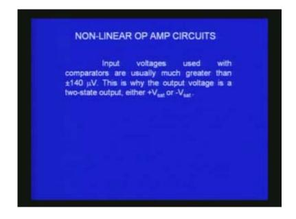
If I have one of the inputs at a particular voltage in this case at zero the other voltage when it goes plus or minus 140 microvolt the output will go to plus or minus  $V_{cc}$  either +14 or -14. So I can detect two voltages within a range of 280 microvolts or to be precise plus or minus 140 microvolts. That is the basic principle of the voltage comparator. In this case one input is connected to the ground; this is the zero.
