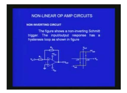
$-V_{sat}$  and  $+V_{sat}$  you get and the UTP, LTP in non-inverting will be  $R_1$  by  $R_2$  times  $V_{sat}$  and  $-R_1$  by  $R_2$  times V saturation.
