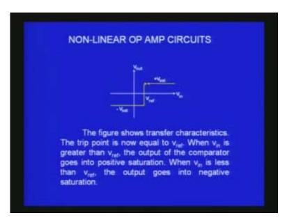
The transition happens at this 1.2 volt or 1 volt or whatever may be the reference depending upon the  $R_1 R_2$  value that you have chosen. You can also have a very similar circuit. Instead of  $+V_{cc}$  I connect the minus. Then what happens? The reference becomes negative voltage. When the reference becomes negative voltage correspondingly the
