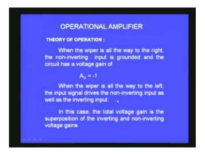
In that case the total voltage gain is a superposition of the inverting and non-inverting voltage gains. Let us try to look at that. We have already seen that earlier in the beginning also. The non-inverting gain is 2 the inverting gain is -1. Therefore total gain is 1.
