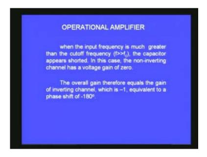
The over all gain is equal to the gain of the inverting channel which is -1 and the minus shows that there is a phase of 180 degrees.
