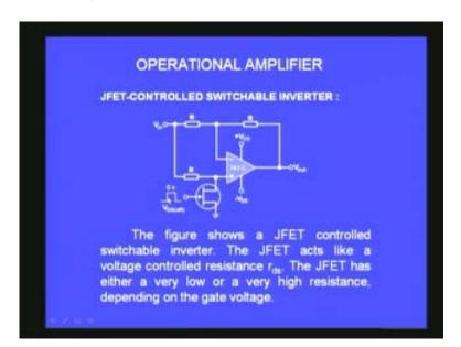
The pulse is from 0 to 6 volts. When it goes from 0 to 6 volts when it is positive this FET will be conducting and when it is ground it will be non-conducting. The JFET acts like a voltage controlled resistance in principle. Depending up on the voltage you apply at the gate the resistance between the drain and the source can be very low or very high. What
