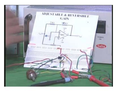
I have taken the multimeter and connect it at the pin number 6 with this circuit wired here. What will be the output? Because the potentiometer is in the minimum position the gain now is 1.01. 1.01 is what you measure at the output voltage of the multimeter.
