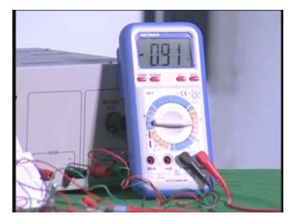
I have changed from +1 to -1 continuously the gain by changing the potentiometer from zero value to a maximum value. This is what we call a sign changer. We can change the sign of the amplifier by continuously varying this from -1 to +1 or +1 to -1 by using the potentiometer. This is again a very simple and useful circuit for applications.
