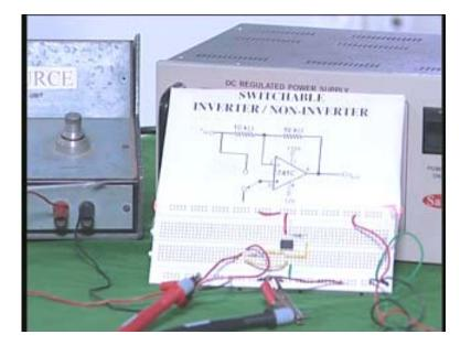
I have now switched the yellow wire from ground to the input terminal and I am now monitoring the input voltage using the same multimeter. I want you to see the multimeter. When you look at the multimeter the multimeter shows 1.02 volts.
