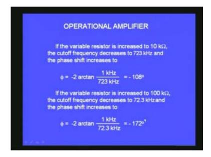
By changing the potentiometer, the RC value, R value the phase angle can be varied by a whole range from almost zero to 180 degrees. I will show you the demonstration of this phase shifting amplifier.
