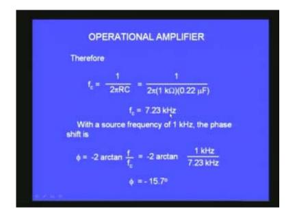
When I have about 1 kilo hertz the phase shift will be 1 kilo hertz by 7.23 kilo hertz that is -15.7 degrees. If I increase to 10 kilo ohm then the corresponding phase shift can be calculated because the cut off frequency will now vary to 723 kilo hertz and 1 kilo hertz by 723 will become 108 degree and when I change to 100 kilo hertz then it becomes 72.3 kilo hertz and the phase angle is 172.
