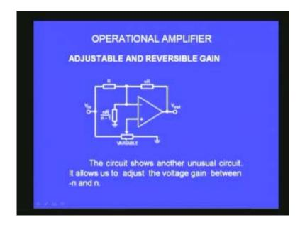
When I put it at this extreme end I will get a gain of -10 because nR by n minus n and when I put the potentiometer to the left extreme on the screen then the gain will be +n. That this +10. I should have a gain of -n to +n as I vary the potentiometer in the circuit. This is what I want to demonstrate to you now.
