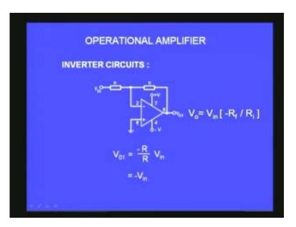
The three is grounded. This is the first part. We applied input; it is only at the inverting input and the gain is R by R therefore it is 1. But because it is inverting we have a negative sign. -R by R times  $V_{in}$  is the output voltage.  $V_{o1}$  I call it because it is a first configuration and it becomes  $-V_{in}$  or if I want to look at it as gain  $V_{o1}$  by  $V_{in}$  is equal to -
