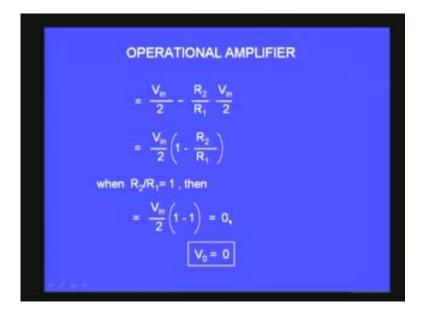
The minimum gain is 0 and whatever is the maximum gain you can get  $-R_2$  by  $R_1$  when you have only the inverting amplifier. You can vary the gain of this amplifier from  $-R_2$ by  $R_1$  to 0. The total voltage gain of this amplifier can be varied over a range by using this type of a configuration. This may be another useful circuit. I will show you demonstration of the circuit also.
