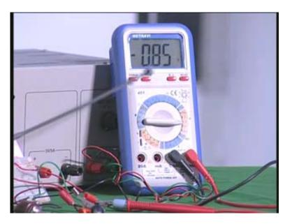
That is the output voltage. Let us see what is the input voltage? I will vary the multimeter connection and connect it at the input. If you look at the multimeter it is +0.84.
