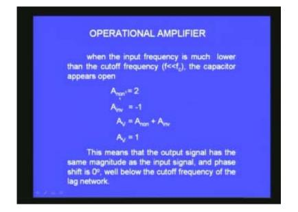
In that case the total gain is due to both inverting and the non-inverting and  $A_v$  is equal to 1. This means that the output signal is having the same phase or zero phase with reference to the input and the gain is 1. When the input frequency is much greater than the cut off, f very, very large compared to  $f_c$  the capacitor appears shorted and in this case the non-inverting channel has a voltage gain of zero.
