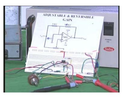
I have nR is 10K. The R is 1K. Therefore n is 10. This is 10K resistor; this is 1K resistor and this is n by n minus 1 times R and because n is 10, 10 by 10 minus 1 is 9. 10 by 9
