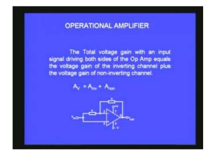
$A_v$  the total voltage gain is equal to A inverting plus A non-inverting. That is what we want to look at. That is what I was just mentioning to you by using superposition theorem. Let us see in more mathematical terms how it is?
