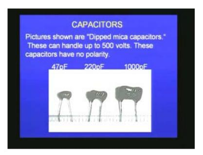
47 picofarad, 220 picofarad and 1000 picofarad are available. You also have metallized polymer film capacitors. They are much more rugged; they have no polarity and the figure shows such metallized capacitors.
