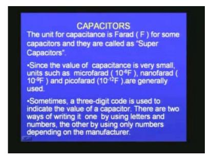
These are the scales that normally we use and we also use similar to the resistors a three digit code which indicates the value of the capacitors or some times they put in terms of
