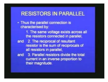
Another very important point with reference to resistors when connected in parallel is that the effective resistance of such a parallel combination will always be smaller than the smallest of the resistors that we have used in the combination. For example if I use 1K in
