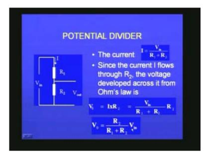
So this is a concept of the potential divider and I have given some examples. If the two resistors are equal then  $V_{Out}$  will be  $V_{in}/2$ ; that we have already seen; equal resistors divide voltage equally.
