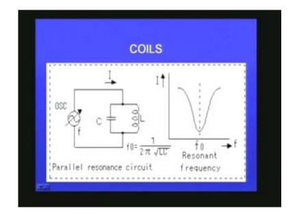
It produces an opposing back EMF that again charges the capacitor and so this goes on and on till all the energy is lost and this is the graph corresponding to the resonance circuit which is shown.
