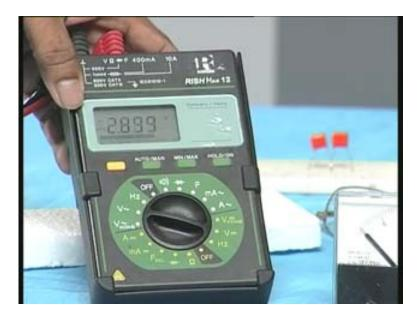
Therefore total 6V is divided among the two resistors connected in series and therefore the concept that same current flows through both the resistors and series resistors divide voltage is very well understood by doing this.
