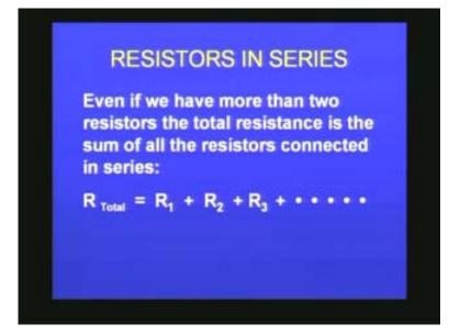
So if I have only 1000 ohms it is always possible that you can combine them and get the value of resistors which is larger than any of the value of resistors that you have for example 1000 ohms. You can easily form for example 3000 ohms resistors by combining three 1000 resistors in series. Like that, you can have any value larger than the value that you have. I just mentioned how this happens. Let me just explain to you how this could be understood in a very simple way.
