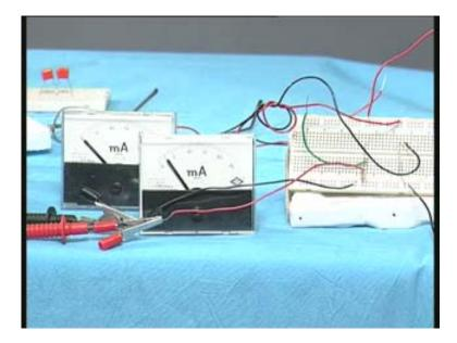
That means two, 1000 ohms connected in series is equal to one 2200 ohms nearly 2000 ohms resistor. Therefore the combination of resistors, when I connect them in series is just obtained by summing all the resistors. That is want I wanted to show you.
