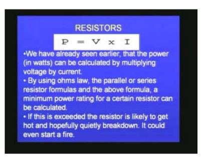
If you use a resistor which has got a lower power rating then the resistor will go back when you connect them in series due to the heat dissipated or it could also start a fire. Next this is about the voltages combinations in series and parallel. I will quickly go over to the experiment and show you the different ways of connecting the resistors in parallel and series and then let us try the experiments.
