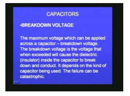
But if I am going to operate the capacitors in regions where the voltage could be as high as 1000V or 2000V then I should buy capacitors with very large break down voltages of the order of 5K or 10K, etc.
