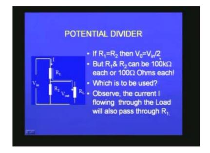
I also mentioned to you in the potential divider that the current flows through  $R_1$  and therefore one has to choose carefully the value of  $R_1$ . We can also have the two resistors replaced by a variable resistor if necessary; that is also possible. And then the last point which is very important in potential divider is with reference to power dissipation.
