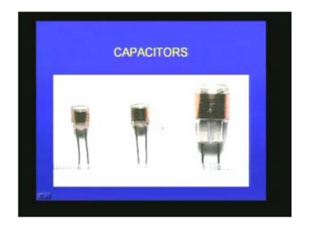
The nice brown color is due to copper being used as the electrode material. Then you have electric double layer capacitor which is called a "super capacitor" and the value of the capacitance is 0.47 farad. You should remember it is not micro farad; 0.47 farad. That means it is a very large value of capacitance. I will show you the picture. You can see here this is very large capacitor which has to be very carefully handled.
