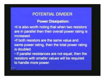
We should always use resistors which are not too small, resistors which are not too large but some thing in between. May be about 1000, 2000 ohms will be reasonable value of the resistors to be used in serial combination for obtaining potential dividers. I will just give one or two simple ideas. Four identical quarter watt resistors, 0.25 watt resistors can be wired in parallel to give a resistor of  $1/4^{\text{th}}$  the value in ohms but four times the power
