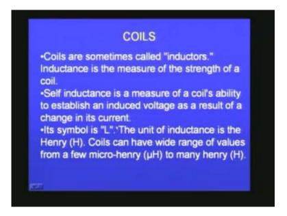
The symbol is L for inductance and the unit is Henry; usually we use micro Henry and milli Henry as units. The characteristic of the coils is that when current attempts to change then there is a reactance. In the case of capacitors whenever voltage changes there
