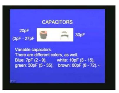
I have shown some more variable capacitors here. It is a ganged capacitor in the olden day radios, which makes use of these.
