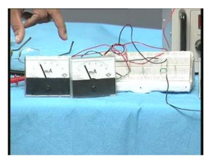
So we can see that parallel resistors divide current and they have a same voltage. That is what I just wanted to show you. So we have seen the actual demonstration of the series and parallel combinations of the resistors. Now we will move to the next component, which is capacitor.
