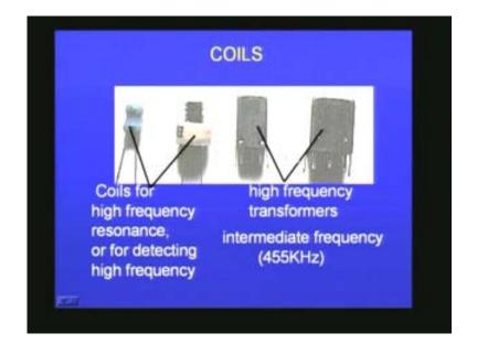
So you can adjust the value of inductance by using screw driver and vary the inductance value.
