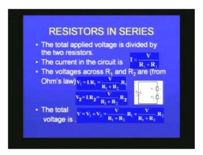
If you see on the screen, the total applied voltage is actually divided by the two resistors  $R_1$  and  $R_2$ . How is that? We can have a look at that. All that we need to know is the simple law of ohms. So now you can see what is the current in the circuit that I showed you? I have given that circuit once again in this frame. You can see there is a battery  $R_1$
