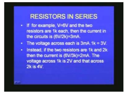
So the voltage across the resistor  $R_1$  which is 1000 ohm is 3V. By the same reasoning you can immediately guess the resistance across the second resistor which is also 1000 ohms will be another 3 volts. So the total voltage therefore will be 3+3, 6V which is the voltage of the power supply and therefore you can see the total voltage of the power supply which is in this case 6V is divided equally by the two equal resistors 1000ohms each.
