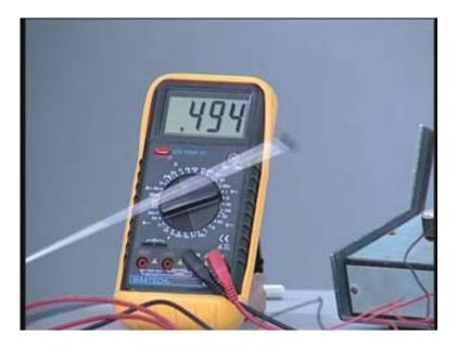
That means this gives around 500 millivolts or about 0.5 volts. Now I take it out and connect this at pin number 6 and find out the output voltage. The output voltage is - 400; about 400 millivolts when I give the input at this point after the resistor. What I do is I will take the input and give it at pin number 3. I have actually given the input at this point at pin number 3 directly. I have given the input from the millivolt source at this point pin
