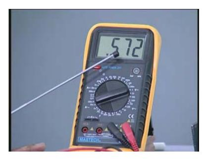
It is not exactly half but very close to half and that shows that whatever resistor I have connected here is approximately equivalent to the input resistance. Actually if you look at
