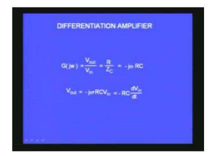
The V output is - j omega C RC into V<sub>in</sub> from this equation and that is equal to -RC dV<sub>in</sub> by dt because - j omega V<sub>in</sub> is nothing but the differentiation of a input signal dV<sub>in</sub> by dt. The dV by dt is nothing but I by C; current divided by C.
