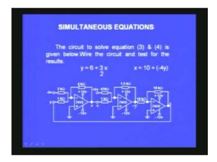
For example I have used the  $V_s$  the reference voltage to be -5 volts and I have used 2K resistor here, 4K resistor here in this first amplifier. If I have only this input what is the gain of this? The gain of this is 4 kilo ohms divided by 2 kilo ohms with a negative sign
