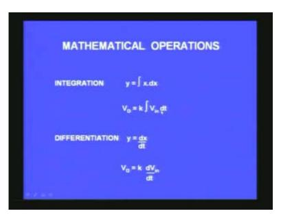
We saw some examples of these. We also saw a demonstration. Today we will discuss on the differentiation circuit where output voltage is going to be some constant multiplied by the time derivative of the input voltage  $dV_{in}$  by dt. V output is equal to k times  $dV_{in}$  by dt. How do we do that?
