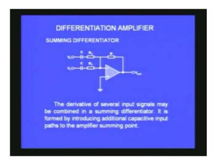
It is a sum of two terms. Each of the term will correspond to the differentiation of the  $V_1$  signal and the  $V_2$  signal and that is what I will get. You will have the summing as well as differentiation perform on the signal. Similarly I can also have another differentiating circuit where I have used both the input terminals. The non-inverting terminal and the inverting terminal both of them are used here.
