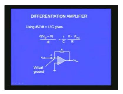
Here at the input side the differential voltage is  $V_{in}$ -0. This is zero here. This is  $V_{in}$  by dt is equal to 1 by C zero minus V output by R at the output and that is also the same as what we have already seen. If you look at the frequency response curve it will be something like this. It is because it is a superposition of two curves. One is due to the op amp about which I have not yet discussed. But I will discuss at some detail later on.
