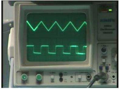
There is of phase factor which you are not able to exactly see but the triangular wave becomes the square wave when I apply through (or) from? a function generator. I also mentioned to you what would happen if I apply a square wave at the input of the
