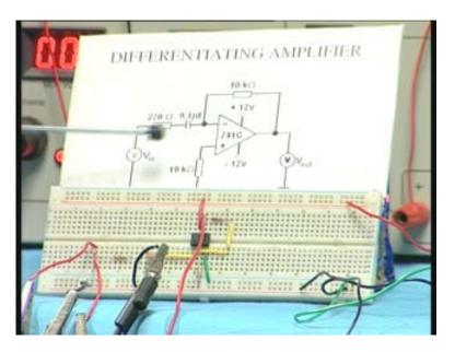
You have an input which is actually obtained from this function generator which can be varied in frequency. You have a sine square triangular wave etc all those outputs are there. These knobs are for applying different frequencies. I have right now applied 1 kilo hertz. I have pressed this button. It corresponds to 1 kilo hertz and this measures approximately the amplitude which is about 200 millivolts.
