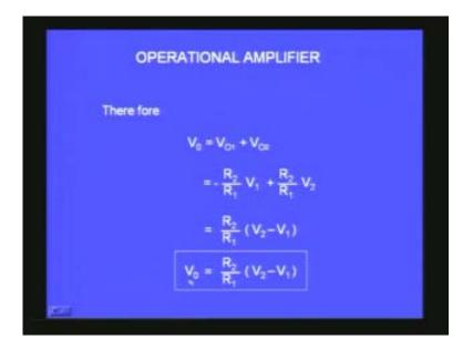
V output is equal to  $R_2$  by  $R_1$  times  $V_2$  difference  $V_1$ . If  $V_2$  is larger than this should be positive and the output voltage will be positive. When  $V_2$  is less than  $V_1$  then you will get a negative voltage here and the output also will become negative.
