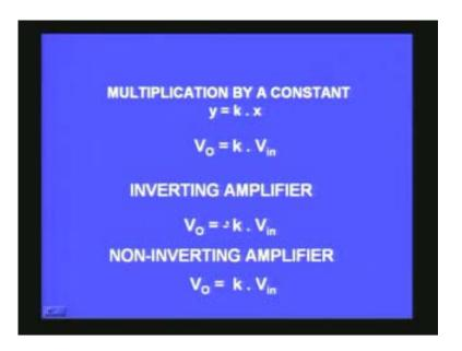
Non-inverting amplifier also can go as an amplifier which will perform multiplication by a constant. That I already mentioned to you. V output is equal to k times  $V_{in}$ . Because we discussed this non-inverting amplifier already let me take the example of the inverting amplifier and show you a very simple circuit which will perform this inversion.
