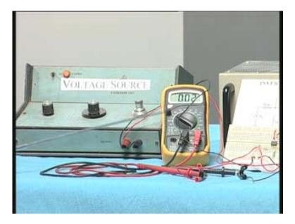
0.02 means 20 millivolts. If you multiply by 1000 you will get it in millivolts. 0.02 if you multiply by 1000 it is 20 millivolts. 20 millivolts multiplied by 10 should be 200 millivolts and what I get in this power supply is 0.20 volts. That means 200 millivolts.
