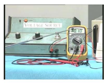
What should be the output? Because there is no  $R_1 R_2$  the feedback is complete; 100%. Therefore the output is also the same as that. Instead of 0.1 it is 0.09 because it is exactly not the same as the input; slightly less.
