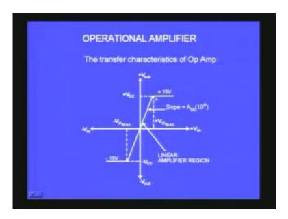
When the input voltage goes beyond the maximum voltage namely about 200 microvolts, the output becomes saturated because of the large open loop gain of nearly 10 to the
