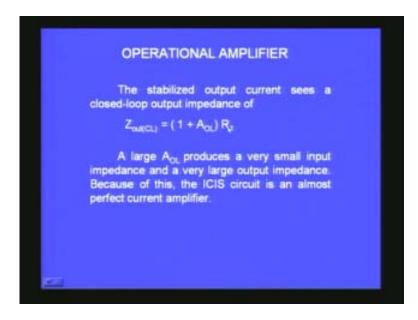
$R_1$  is a normal thing that you will get is multiplied by this large number. Therefore output resistance effectively is increased and the output acts as if it is a current source. That is
