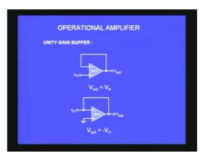
In one circuit the output is completely connected to the input without any resistor. There is no resistor. Output is connected to input and the input voltage is now given to the non-
