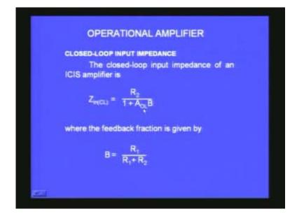
Because the feedback fraction is given by beta is equal to  $R_1$  by  $R_1$  plus  $R_2$  that is the ratio of the fraction of the output which is fed at the input and the effective input resistance is going to be less now. A beta is a large value. So  $R_2$  divided by A beta can be very, very small. The effective input resistance is reduced. Similarly if you look at the output resistance of the closed loop configuration it will be multiplied by the factor 1 plus  $A_{OL}$  into  $R_1$ .
