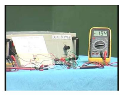
Whenever I increase the input voltage the output voltage is always negative. That shows it is an inverting amplifier. The positive voltage is converted in to negative voltage. These two points are to be borne in mind. Having seen the inverting amplifier now we can also see a small variation of the inverting amplifier and the variation of the input inverting amplifier is a very, very useful circuit which is useful in many buffer applications. For example I have shown on the screen two circuits.
