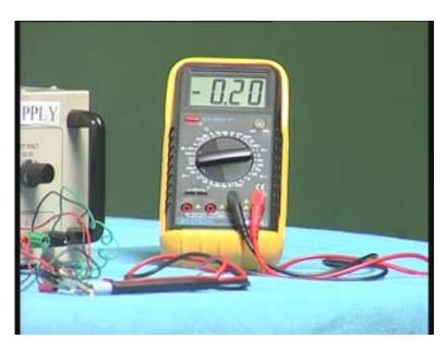
0.02 is coming as 0.2; multiplied by 10 times. If I put 0.3 here, 30 millivolts you get 0.3 volts at the output correspondingly. If I make it 40 millivolts, 0.04 and the output voltage
