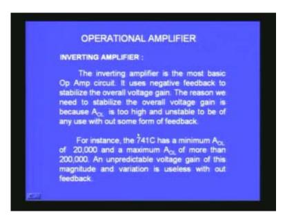
In many of the books inverting amplifier will be given as the first circuit; most basic circuit in the op amps. Because you also have here negative feedback, the negative feedback stabilizes the performance of the amplifier. When you have negative feedback the amplifier performs much more reliably. Because the open loop gain can be different
