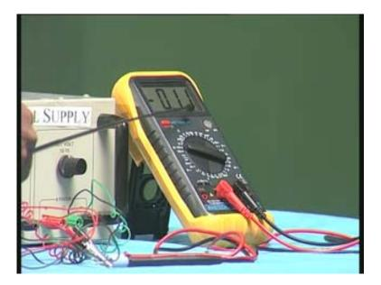
It is exactly multiplied by 10 times with reference to the input current. I am going to change this dial to 20 microamperes and you see what the input current meter reads. It reads 0.020 which is actually 20 microamperes.
