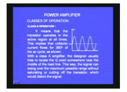
In a class A amplifier the collector current flows for all the 360 degrees of the ac cycle, full cycle. You have another class of amplifiers which are called class B amplifier where you try to choose the operating point far away from the midpoint, towards the lower end for example.
