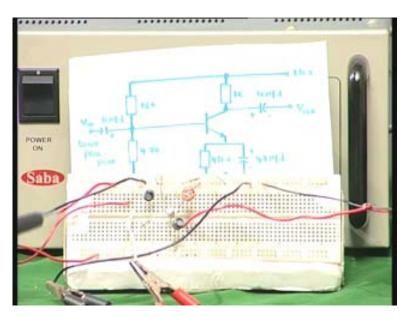
This is the power supply. You give about 5.5 volts or about 6 volts here and the power supply is connected to bread board and this is the signal source that is connected to the input and the output is monitored on the oscilloscope. Now you can see there are two sine wave traces that you see on the screen.
