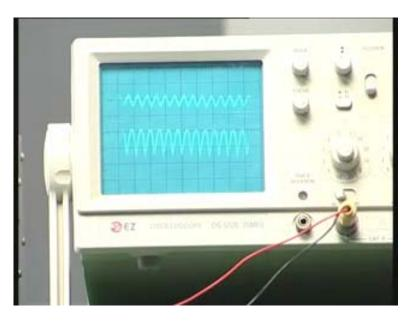
Now I increase the frequency still further. Now let me change the sweep frequency so that you can see one or two waves again. You can see the gain is almost same. As I increase the wave form is only shrinking but the amplitude is not changing as you can see that.
