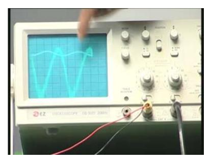
You can see that. This amplification comes around some frequency which we can identify here. It is around 100 hertz I have kept here. You can see this is 100 hertz. Let me increase the frequency. You can see in the oscilloscope as I increase the frequency the amplitude keeps increasing. It was previously very low now it has increased. Let me reduce the gain factor and I will keep increasing the frequency and it is almost constant now.
