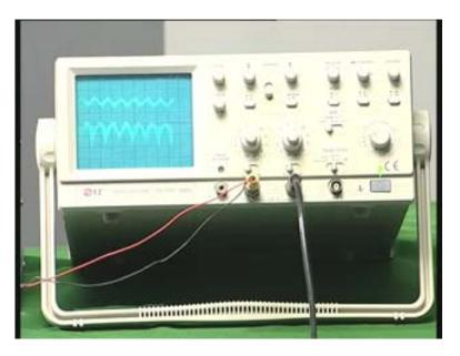
Now I will change the range from 100 hertz to 1 kilo hertz and you see again the amplitude is relatively larger for the output compared to the input.
