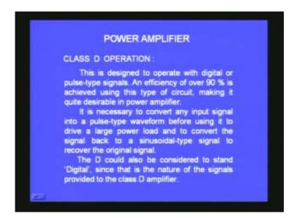
When you use digital signals you try to make use of amplifiers which are operating in class D mode and the efficiency of the class D mode is more than 90% and they are very, very useful in digital amplifier circuits.
