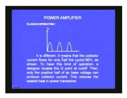
That means the collector current will not be flowing for the full 360 degrees but it will be only flowing for about 180 degrees. If it is exactly on the x-axis it will be 180 degrees. To have this kind of operation a designer will locate the Q point at the cut off; that is the most important point. If I bias it at the Q point at the Q cut off then only one half of the
