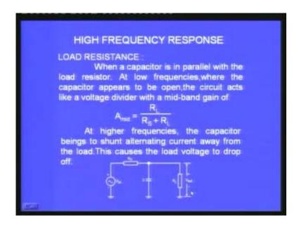
That is all the difference. With the  $R_L$  and  $R_s$  combined in the actual circuit the  $R_s$  and  $R_L$  will come in parallel.
