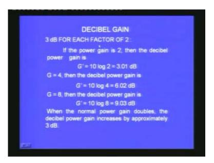
For every factor of two the power gain will increase by a value corresponding to 3 dB. That also can be obtained from the same formula G prime is equal to 10 log 2 that is 3 dB. If it is 4 it will be 6 dB and if it is 8 it will be 9 dB etc. For every factor of 2 the
