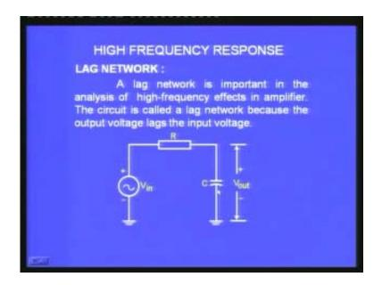
Now we are taking the output across the capacitance and not the resistance. If I have the frequency response of such a network it will just be the other way. That it means it will be high initially at low frequencies and it will fall at very high frequencies.
