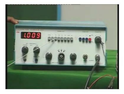
That means it is 1 into 10 about 10 hertz that is at a very low frequency. At very low frequencies the gain should be very, very low. That is what we saw. Let me quickly go to the next stage. That means I am pressing the 100. Now I am in 100 hertz frequency and now if you observe the oscilloscope you still have large amplitude for the input but the output is still very, very low.
