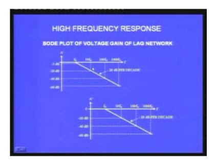
If it is hundred times the cut off frequency it is -40 dB. If it is 1000 times the cut off frequency it is -60 dB. It is constant for sometime and then it starts falling below. This slope is 20 dB per decade. That is what we call this. This variation it is falling by 20 dB
