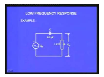
The lead network becomes important at the low frequencies and that corresponds to the coupling capacitors. The coupling capacitors are like this if they go into the base of a transistor amplifier here. The coupling capacitors are the ones which are to be very carefully analyzed for looking at a low frequency cut off amplifiers and similarly for the high frequency you will write ..... are all the contributing factors.
