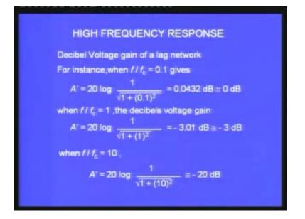
If I go in multiples or octaves there is a change of about 6 dB in voltage gain. So these are exactly same. I have given some examples here and then I will show you the graph corresponding to the Bode plot, log log scale of the voltage versus frequency of the lag network. At  $f_c$  the gain will be zero. Then if I go beyond  $f_c$  by 10 times you would find you have about -20 dB. It starts falling; minus means loss not gain.
