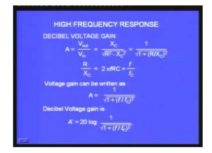
This is what previously I called  $f_1$  and  $f_2$ . This is actually corresponding to  $f_2$  the previous lead network corresponds to  $f_1$ . Here I generally call them as cut off frequency therefore  $f_c$ . The rest of the discussions are very similar. If I go in decade in voltage gain there is a 20 dB variation in decibel.
