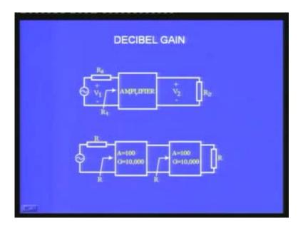
$V_2/V_1$  is the voltage gain.  $R_1$  and  $R_2$  will be matched. Usually the input resistance will be matched. When you go into the overall voltage gain you should try to add the decibel voltage gains of individual amplifiers. That's what I wanted to show here.
