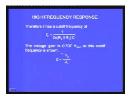
The frequency response of an amplifier is normally represented on a logarithmic scale.
