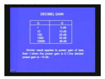
Similar results will apply to power gain which is not actually the gain or loss which are less than 1. When the power gain is 0.1 the decibel power gain is -10 dB. When the power gain is -0.01, that is 100 then it will become -20 dB etc. Similarly we can also look for what happens to the power gain when it is a factor of 2.
