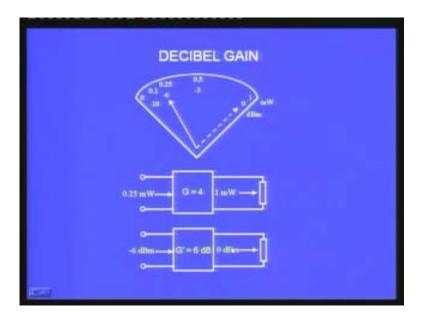
When will it become zero? Only when I add - 6 to + 6. The gain of the amplifier in decibel is 6 dB and that is also the same as in ratio a factor of 4.
