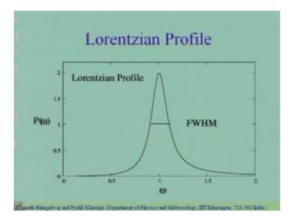
We expect the frequency response of the speaker, the power that is dissipated away and the power that is put into the sound wave by the speaker, we expect that power that is drawn from the music system, we expect that to be have a Lorentzian profile, from what we have an from analysis, we expect that to have a Lorentzian profile. And we know that, the width of the Lorentzian profile is 2 beta.
