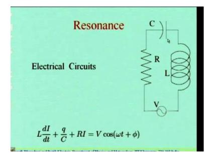
So, the circuit which we are going to analyze which we are analyzing; the L C R circuit connected the L C R elements connected to an, to a voltage source this circuit can also be analyzed if, we talk in terms of the impendence. So, just like if I had only a resistance
