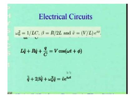
By exactly the same equation as that of a damped simple harmonic oscillator, with an external force, the external force here is the voltage that is, generated by the voltage generator. And here the resistance plays the role of the damping element, the inductance plays the role of the mass and the capacitance plays the role of the spring. So, with this identification, we can analyze the L C R circuit couple to a signal generator, in exactly the same way.
