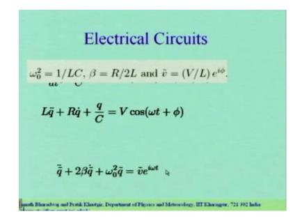
Now, this equation which governs the circuit can be written fully in terms of only the charge. So, the current we know is; the rate of change of charge, the rate at which charge flows in the circuit. So, we can replace this term over here with R into q dot where, q dot is the type derivative of the charge and we can replace this term with L into a second derivative of the charge. So, the same equation can also be written in this fashion.
