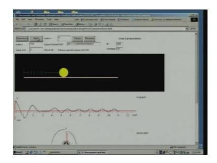
So, here we have cross resonance. So, we have cross resonance and we are driving the oscillator at a force, whose frequency is considerably larger than the resonant frequency. So, you have these transient oscillations at the natural, I think we could increasing damping, the damping here is too small that, transience will continue for a long time. So, let us increase the damping to 2 B has a value 2.
