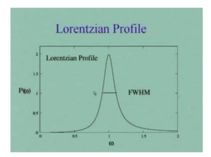
So, the average power drawn by this circuit is follows the Lorentzian profile. It has a peak at the natural frequency omega naught and then, if you drive it at other frequencies, the power that is dissipated and the resistance false off. You could calculate the full width that half maxima of this peak, for low values of the damping coefficient where, beta is much smaller than omega naught, the full width that off maxima is twice approximately twice beta.
