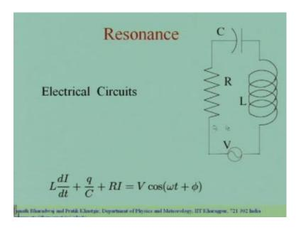
So, you can apply Ohm's law to the circuit and say that the voltage across this, should be equal to the voltage across all of these elements combining together, these elements are in series. So, you can add up the impedance of all of these 3 elements. And the impedance across this is that, the current into the, voltage across these 3 elements is the current into the impedance.
