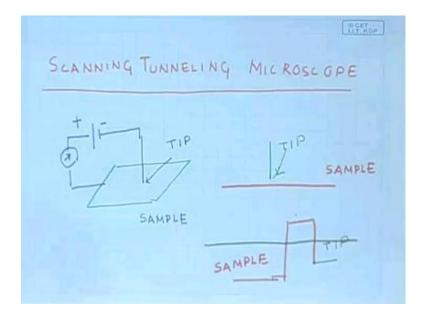
Now what is done in the scanning tunneling microscope is that, the tip is moved up and down, as it scans the tip is moved up and down automatically by a feedback loops, so as
