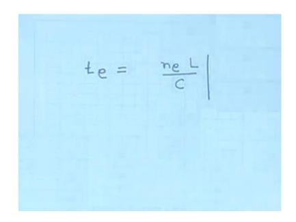
So, for the extraordinary polarization when electric field is along the optical axis the time the light will take is going to be ne L by C or if you ask the question what is the optical path?
