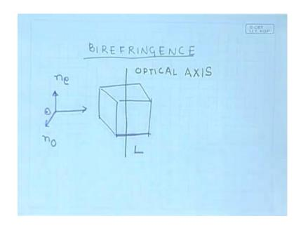
So, quarter wave plates are crystals like this where the length has been adjusted. So that the optical path difference between this polarization and polarization between these 2 is lambda by 4.
