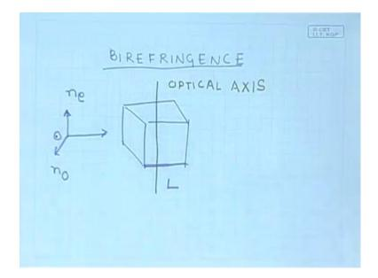
Let us ask the same question for the situation where the electric field is perpendicular to the optical axis. So, when the electric field is perpendicular to the optical axis the refractive index is no.
