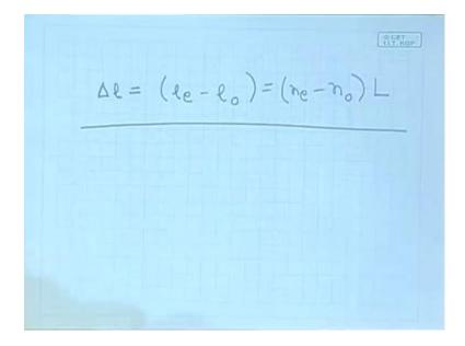
So, the difference in the optical path for 2 different polarizations is le minus l o. Well, this could be positive or negative we are not really interested in sign we are interested in just the magnitude. So, this is going to be the difference in the refractive indices divided by into the length of the crystal. This has got several applications let me for example, you could make water called quarter wave plates.
