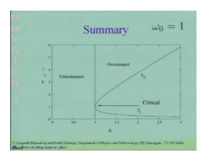
So, if you would like a, like your door like to design your door shutter. So, that it shuts in a reasonably small time then you should choose the value of beta to be close to the critical damping situation. The critical damping situation, the situation when you have critical damping is the 1 which corresponds which where the situation will come back to the equilibrium position to come back near the equilibrium position the fastest.
