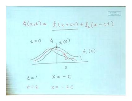
So, this very special solution where this is a sin function, but in principle it could be any arbitrary function provided it is well behaved at infinity well behaved everywhere and it is differentiable everywhere. So, these were the plane wave solution to be wave equation now let us we will discuss another kind of solution today. So, the other kind of solution that we are going to discuss is what is called as spherical wave solution.
