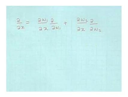
So, del del x is equal to del w1 so, the derivative with respect to x the partial derivative with respect to x. You can express in terms of partial derivatives with respect to w 1 w 2 using the chain rule of differentiation and. So, you have to now calculate these derivatives the derivative of w 1 with respect to x and derivate of w 2 with respect to x. (Refer Slide Time: 16:17)
