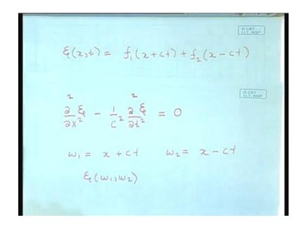
So, we have obtained the most general plane wave solution to the wave equation plane planar solution to the wave equation.
