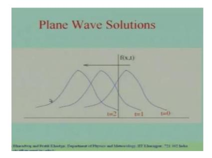
So, this picture over here shows you the evolution of the left propagating plane wave solutions. So, this is the solution at t equal to 0 at t equal to 1 the whole solution has shifted to the left and at t equal to 2 it has shifted further to the left the shift being. So, from here to here shift is going to be c from here to here shift is going to be 2 c and at t equal to 3 it could have shifted to 3 c.
