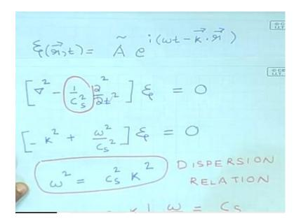
So, this is need a solution to the wave equation provided the wave number k the wave number corresponding to this wave vector and the angular frequency are related in this fashion. So, the relation between the angular velocity and the wave number is called the dispersion relation. So, provided the angular velocity and the wave number satisfy the dispersion relation corresponding to this particular wave. So, the dispersion relation for
