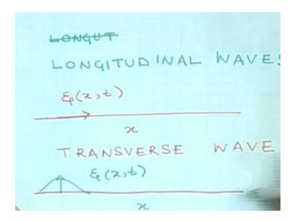
So, we have different kinds of waves possible we have longitudinal waves possible. We derived the wave equation for a longitudinal wave which is disturbances in an elastic medium, longitudinal disturbances in an elastic medium. But you could also have transverse waves like the disturbances in a string now in all such situations.
