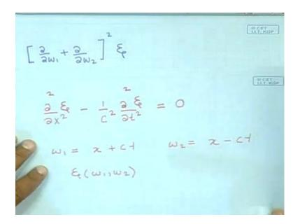
So, what we have done is we have written this wave equation in terms of derivatives with respect to w 1 and w 2. This is the derivative with respect to x which has been written like this is the derivative to the respect to t divided by c square, the second derivative
