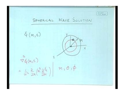
You have to represent this Laplacian operator in terms of derivatives not in terms of x y of x y and z, but derivatives in term of with respect to r theta and phi.
