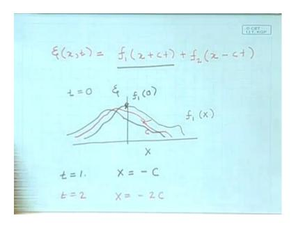
It could be some arbitrary function f 1 of w 1 and w 1 is x plus ct plus some other arbitrary function f 2 of w 2 which is x minus ct. And this combination linear superposition of 2 such functions is solution to the to this wave equation which for which you are trying to find a solution.
