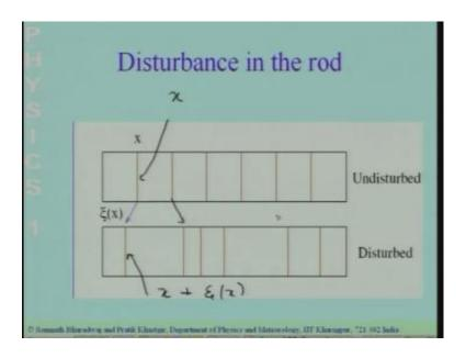
And, because of the disturbance that, we have introduced possibly be a by taping it at one end and whatever means, these lines have got moved around and the different elements have got compressed or verified. So, let us now, focus our attention on the element over here. So, I have drawn the line on the element over here, after the as the consequence of the disturbance. This gets shifted to a new position and the deformation
