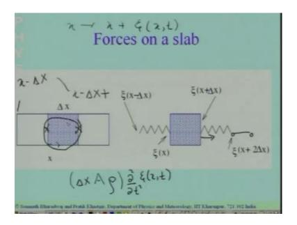
The force on the from the right hand side involve the derivative at this point. To calculate the total force on this mass element, which we are focusing on, we have to add up both of these.
