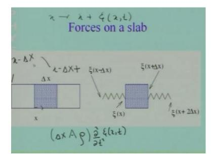
So, this is the element that we have replaced by this spring its undisturbed length is delta X.
