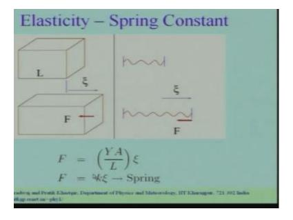
So, it tell us the constant relating the force, which develops, if I deform this object by a by a length xi, this constant is the Young's modulus into the cross sectional area divided by the undeformed length of this object. So, the point, which I am trying to make over here, is that, we can an elastic material. This is an elastic rod of cross sectional area A
