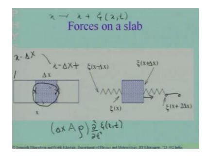
So, the total force due to the 2 elements on the 2 sides.
