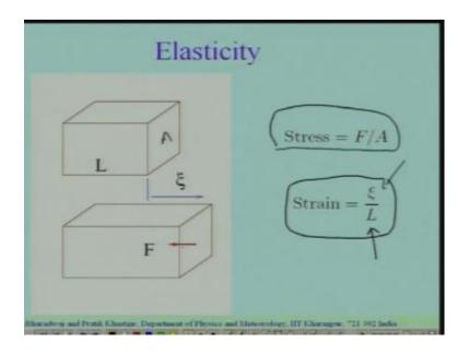
So, let me recapitulate briefly, what exactly do? We mean by elasticity. So, this picture shows you a bit of an elastic medium the cross sectional area of this medium is A. So, this is the cross sectional area of it is, it is A and the medium the elastic substance that we are interested in has a length L length L cross sectional area A. Now, there are 2 quantities, which are defined in elasticity one is called the stress and the other is called
