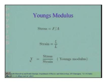
And for an elastic substance the ration of the stress force by unit area and strain is a constant, which dependence only on properties of the material. So, depending on the material, it wills the ration of the stress divided by the strain. The stress divided by the strain will be a constant call the Young's modulus and this is a property of the material
