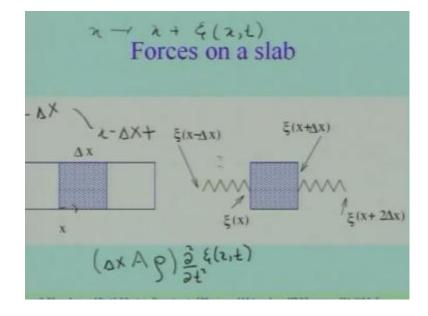
The left tip of the spring gets, displaced to xi x minus delta x the right tip get this, displaced to xi x by an amount xi x. So, the deformation of the spring is the difference between these 2 and there is going to be force, which is going to be opposite, it to this deformation, which is the force due the spring on the left which is what I have shown over here.
