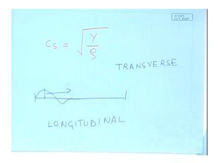
So, for an elastic wave the phase velocity Cs in the medium is equal to square root of the Young's modulus divided by rho the density of the medium. And if I have the different kind of wave in a different context then, they then the wave equation is usually going to be just the same as this.
