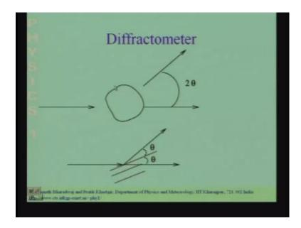
And so, you have now, a sample made up of that lanthanum strontium manganese oxide on which you have x-ray. And what you have done is what the diffractometer does is it, measures the intensity of the scattered x-ray. As a function of this angle which is called 2 theta.
