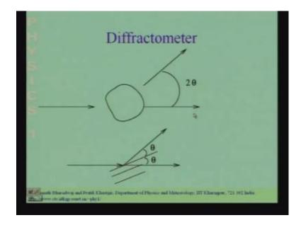
So, you can measure the intensity of the scattered light as a function of this angle, which you can interpret, has been twice the grazing angle with respect to the plains, which have the scattered x-ray in this direction. And what you get is the intensity pattern has a function of this 2 theta from them x-ray diffractometer.
