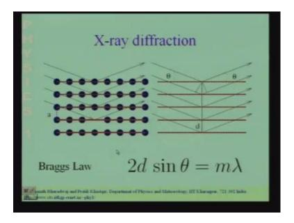
So, what we have over here is x-ray diffraction pattern that is going to produce by the radiation from this periodic arrangement of sources, each atom is going to scatter out
