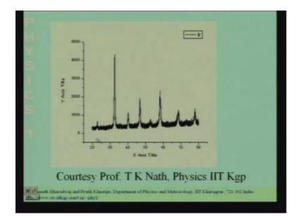
And this shows, you the intensity which is measured at different angles 2 theta. So, x axis as 2 theta, the y axis as the intensity and notice that as you vary the angle.
