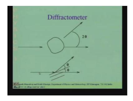
Diffractometer x-ray diffraction incidentally is very useful technique to determine the structure of materials. If I give you a crystal and I do not know, it is inter atomic spacing I do not know, how the atoms are arranged. I can use the diffraction pattern to determine the inter atomic spacing and the structure the arrangement of the atoms inside this crystal.
