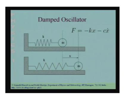
In the last class we had considered the simple harmonic oscillator we had taken the prototype simple as the prototype simple harmonic oscillator the spring mass system shown over here. We had worked out the solution to this to the motion of the particle, if it is displaced from equilibrium and the solution as we had seen in the last class is.
