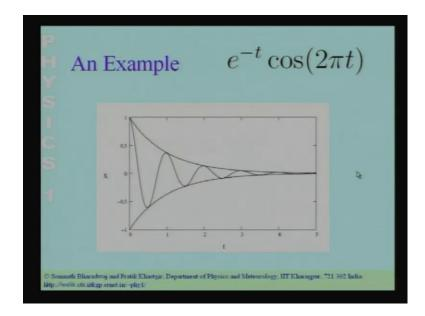
So, let us now have a look at what this oscillation looks like. So, this shows you an example of the under damped oscillations. The particle continues to oscillate just like in the situation where you had no damping here the particle till does oscillations. So, you have these oscillations, but you have this feature that the amplitude of the oscillations
