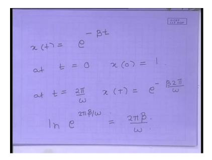
The oscillation the amplitude of the oscillation falls like this at t equal to 0. We have x 0 which is equal to 1 and at after a time period time period is t equal to 2 pi by omega. So, x after a time period will have a value e to the power minus beta 2 pi by omega. You are supposed to take the ratio of this divided by this. So, if you divide this by this you will get e to the power 2 pi beta by omega and then if you take the natural logarithm of this you will get 2 pi beta by omega.
