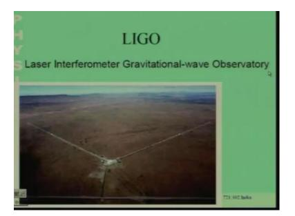
From here jump right into the present times at present there is a very large very large Michelson interferometer experiment going on the arm lengths of the of this particular Michelson interferometer experiment are quite large. The arm lengths are four kilometers in length and this picture shows you the this particular Michelson interferometer. So, this Michelson interferometer is this is this is an experiment called LIGO L I G O laser interferometric gravitational wave observatory.
