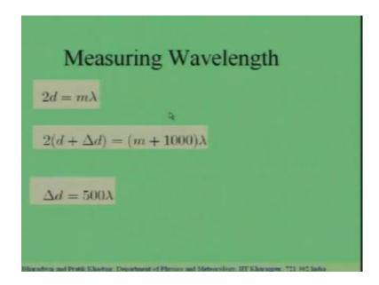
Let me, now discuss some very interesting uses of the Michelson interferometer. 1 very interesting application and quiet useful application of the Michelson interferometer is to measure the wave length of light. The visible light as we have learnt, it has a wave length somewhere around 500 to 600 nanometres.
