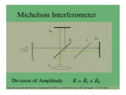
Which, they are produced in this direction. So, they are there will be 2 images of ground glass plate produce in this direction. Which I put my eye here and the eye piece of the telescope I will see 2 images of the ground glass plate 1 arising from the light which is transmitted comes here and is it reflected. Another arising from the right which is reflected and then, transmitted so, 1 produce by M1, another produce by M2.
