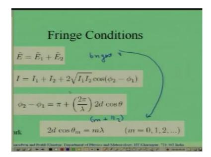
This is the fringe condition. So, if I increase theta maintaining the same distance d. If I increase theta going outwards means increase in theta then, cos theta the value of the cos theta has to will go down cos theta is maximum. When, theta is 0 at the centre now if I increase the theta the value of cos theta goes down. So, you can see the value of m will corresponding go down.
