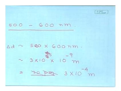
So, delta d is the order of 500 times the wave length of light which is somewhere in a the range of 600 nanometres 500 to 600 nanometres. So, this the order of the 3 into 10 to the
