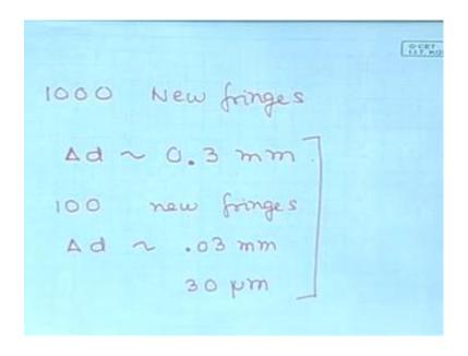
So, delta d for 1000 new fringes at the centre delta d is of the order of point 3 millimeters. If you have 100 new fringes delta d is of the order of 0 3 millimeters, which is 30 micrometers both of these can be measured using a micro meter screw gage.
