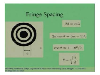
Next, let us ask the question what is the fringe spacing. So, I have already told you that in Michelson interferometer experiment, you will get circular fringes. So, suppose we adjust the interferometer in such a way. So, we adjust 2 arm lengths in such a way. So, that the difference between the 2 lengths is such that is get a dark sport at the centre of the field of view.
