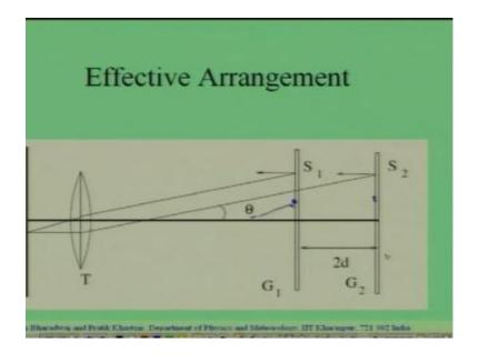
So, this is the role of the lens. Now, let us see what lens does in this particular situation. In this particular situation, we have 2 images of the exactly the same ground glass plate. Let us, look at the image G1 produced by the mirror M1, every point on this ground glass plate acts like a source this is an extended source. So, every point over here acts like a source and every point on the ground glass plate sends out light in all directions.
