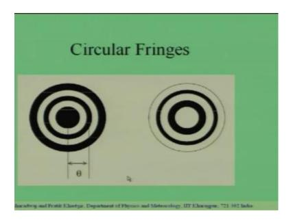
So, what this tells us is at you will get circular fringes. So, the fringe pattern that you observe on the screen over there if you put your eyes at the focal at the eye piece of the telescope or if you put a lens and focus the light on to a screen, what you will observe over there is circular fringe patterns. You will get circular patterns of dark and bright.
