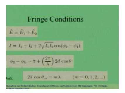
So, this is the wave from the first image this is the wave from the second image both of them will get superposed on that point in the screen. So, I wish to calculate the intensity that point in the screen. So, I wish to calculate the intensity at this point arising from this image and this image together. The intensity at that point is i1 plus i2 plus 2 root i1 i2 cos phi 2 minus phi 1 We have discussed we derive this formula 2 class back and we have discussed it.
