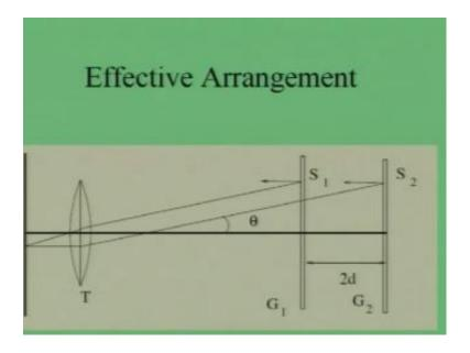
So, the effective arrangement is again shown over here the thing which I was just discussing. So, you have 2 images of the ground glass plate which are produced in the direction of the line of sight.
