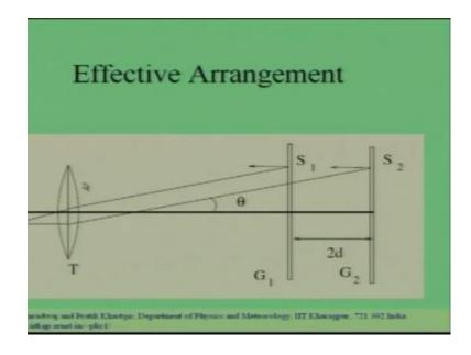
So, i1 is the intensity of light coming from here, i2 is the intensity of the light from here phi 2 minus phi 1 is the phase difference between these 2. And the phase difference between these 2 waves arises because, they have to 1 traverses of different path these 2 these 2 images of ground glass plate are effectively sources which are separated by distance 2d. And if a looking at wave which is emitted at an angle theta then, the path difference between these 2 is 2d cos theta.
