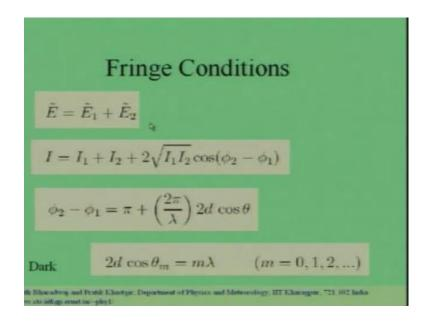
So, let us ask the question what is the intensity pattern on the speed over here going to look like right. So, the intensity patron on the screen over there is going to be the super position of the of 2 waves.
