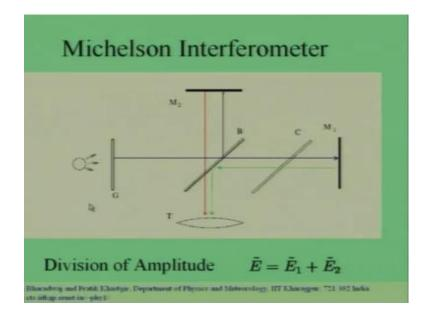
If you follow the beam the wave which gets reflected and then, comes here notice that it undergoes an internal reflection. It undergoes an internal reflection at this over here because, it gets reflected from the interface of the glass and air. Whereas, the transmitted wave undergoes an external reflection because, it is reflected at the boundary of air and the glass.
