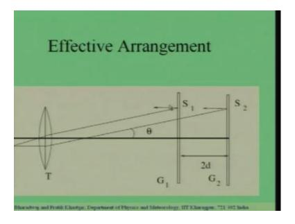
Light which is emitted parallel to the axis over here, theta equal to would be focused to the centre over here. Or if you were to place here eye at the eye piece of the telescope which you add over here. Then, the direction which you see at the centre of the field of you at the corresponds to light which is propagated, which is embittered over here at theta equal to 0. Increasing theta means larger and larger circles over here.
