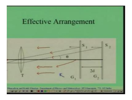
So, now any difference in the position of the images is only due to differences in the lengths of the 2 arms. And the separation between the 2 images of the ground glass plate is exactly twice the difference in lengths of the 2 arms. So, this is the telescope now let us tern a attention to the image this is the telescope. So, we can for our purposes replays the telescope by a lens and put look at, the image of the produce by this lens at the focal plane.
