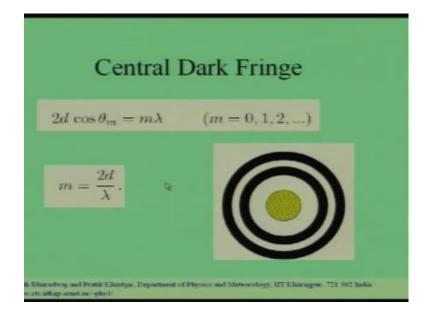
So, this angle over here is theta. So, this is the line of sight theta is the angle over here. And the condition is for dark fringe is 2d cos theta should be equal to m lambda, this will give you a dark fringe of order m at an angle theta m for a bright fringe you can you have to replace this by m plus half.
