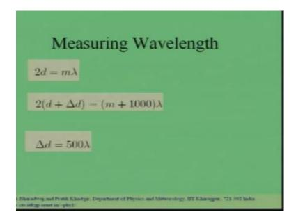
So, you can measure the distance you have to move 1 of the mirrors in a order to produce 1000 new fringes or you could measure the distance you have to move the mirrors 1 of the mirrors to introduce 100 new fringes. And once you can if you can measure this, you can determine the value of the wave length of light lambda. So, delta d is of the order of 500 lambda if you have 1000 new fringes.
