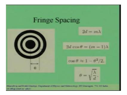
Then, we have a bright fringe around it and then, we have the first circular dark ring. And we would like to calculate the spacing between 2 dark rings. So, let us calculate these distance of the first dark ring from the centre of the central dark spot. So, the central dark fringe occurs that theta equal to 0, it satisfies the condition 2d is equal to m lambda where m is an integer.
