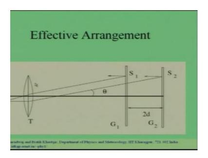
Remember, again is going to be a super position of 1 wave, which originated from this image of the ground glass plate, another wave, which originated from this image of the ground glass plate. We will focus on only 1 point on this image and 1 point on this image. The waves which are emitted at an angle theta from here and here both of them
