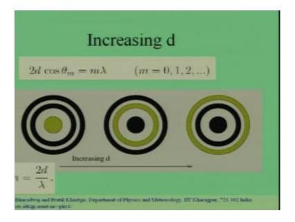
So, that there is a dark spot at the centre. So, I have adjusted the Michelson interferometer. So, that there is a dark spot at the centre. Now, I have already told you that if I increase the difference in the arm length, if I increase the by moving 1 of the mirrors. Then, this particular dark fringe is going to go outwards and a new dark fringe will appear at centre. So, this particular dark fringe now becomes like this bigger and there is a new dark fringe at the centre.
