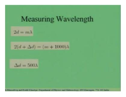
So, the Michelson interferometer gives us a method by which you can measure the wave length of light. So, suppose we adjust the Michelson interferometer.
