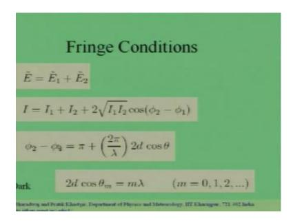
So, phi 2 minus phi 1 will arise because, of this path difference 2d cos theta. You have to multiply by 2 phi by lambda, to get the phase difference between the 2 waves. Now, there is another effect which contributes to the phase difference this effect is as follows.
