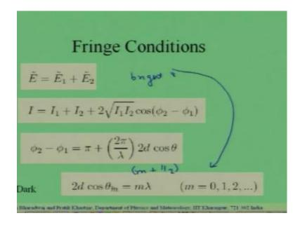
Then, this has to be included. So, the phase difference between the 2 waves is pi plus the contribution due to the path difference. Because, the 2 sources do not, 2 images do not go inside. So, this is the total phase difference between the 2 waves. Now, if this is the phase difference let us, ask the question under what condition are we going to get a minima in the intensity.
