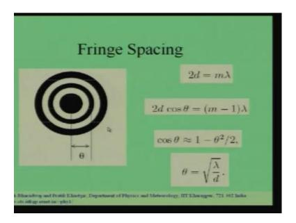
And we have studied various properties of fringe pattern. The fringe spacing, how the fringe pattern evolves if you increase the distance between the 2 mirrors. And then, we studied 1 application of the Michelson interferometer. We studied how you can use the
