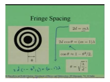
So, for the first the fringe condition for the first fringe tells us, that 2d cos theta is equal to m minus 1 lambda. This is the condition for the first fringe. This is the condition for
