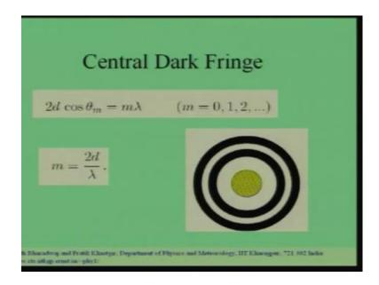
The condition for there to be fringe is 2d cos theta should be equal to m lambda theta is the angle with a line of sight to the centre.
