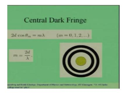
So, suppose we have adjusted the whole interferometer. So, that the central fringe at the centre of the field of view you have a dark fringe. Let me, remind you once more what we mean by the centre of the field of view.
