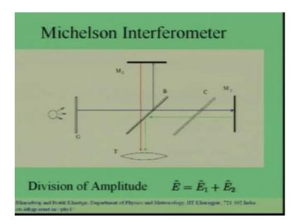
So, in today's lecture we have learnt about the Michelson interferometer. The Michelson's interferometer achieves interference through the division of amplitude. The same wave is divided into 2 waves of lesser amplitude and these are sent to through different paths and then, made to interfere.
