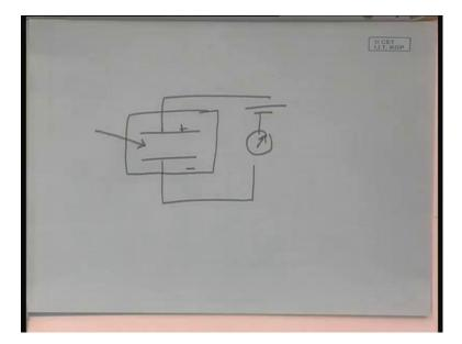
So, what you could do is you could take a cavity, a glass tube or something like that and have to 2 electrodes over here and fill it with some gas. Typically the electrodes are not shaped like this, but for our purposes it does not matter. And you connect it to a battery and an ammeter. So, this gas will normally be neutral and there will be no current
