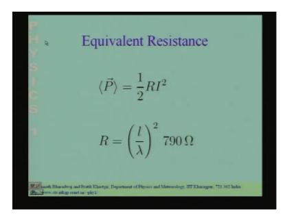
An effective resistance and it can be written as half I square into R where, R is the length of the dipole divided by the wavelength the square of this into 790 ohms. So, we know the value of the amplitude of the current. So, I is known half you have to put a factor of half, what you have to do is to calculate the resistance corresponding to this dipole. To calculate the resistance, the length of the dipole is known. What you have to do is you have to calculate lambda the wavelength.
