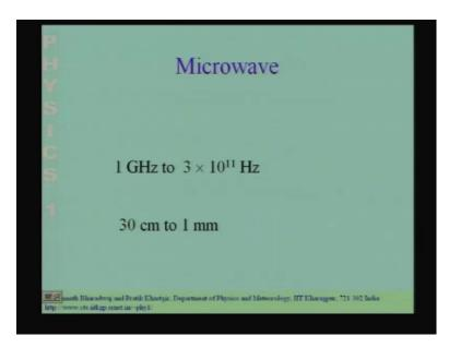
Then, we shifted on to a slightly higher frequency band; the range from 1 gigahertz to 3 into 10 to the power 11 hertz. This is referred to as microwave.
