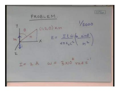
Problem which we will discuss is, we have a dipole which is aligned with the y axis, it is of the origin of the x y z axis and it is aligned with the y axis. The dipole has a length of 1 meter, it is being fed with an oscillating current and the amplitude of this oscillating current is 2 amperes. The angular frequency of the oscillating current is 3 into 10 to the power 6 radians per second.
