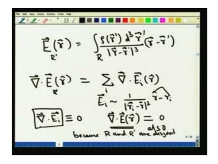
So, please remember this geometry well before I proceed to write the next step. What would be the value of the electric field my electric field? At any given point r in the region r prime. So, let me emphasis that here is simply given by rho of r prime d cubeb r prime divided by naught r minus r prime cubed into r into minus r prime. You people are quite familiar with this result. Of course, r prime belongs to region r that is something that we have to remember.
