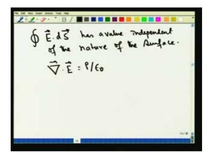
We can conclude that the value of integral e dot d s should be independent of the nature of the surface; it really does not matter whether you take the spherical surface. It really does not matter whether you take a more complicated surface. It is not a property of the surface it is simply a property of the charge that is encloses.
