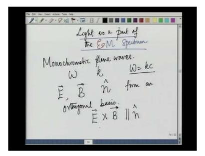
Even more importantly, we found that the electric field, the magnetic field and the direction of propagation, which I shall denote by n, from an orthogonal basis. Of course, I have to replace the electric and the magnetic fields by their unit vectors. Anyway we not only understand that they form an orthogonal basis but we also found that if you fix the direction of the propagation then E cross B, the cross product of the electric field vector, will be parallel to n.
