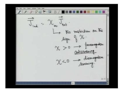
So, with this introduction what I will now do is to write J induced is equal to chi m; everything has something to do with magnetic field; J external. What about the sign of chi? If the material is diamagnetic, chi will be negative; if the material is paramagnetic, chi will be positive. So, no restriction on the sign of chi is that your chi can be greater than 0, in which case I have paramagnetism, why?
