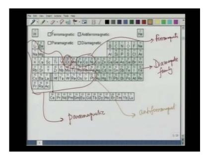
Now, this is a kind of very nice table, which tells you, what the materials, which are paramagnetic. In fact, all the, this is the periodic table, what are the atoms, which are diamagnetic and what are the atoms, which are paramagnetic and we also have atoms, which are anti-ferromagnetic and ferromagnetic, which I will come to later.
