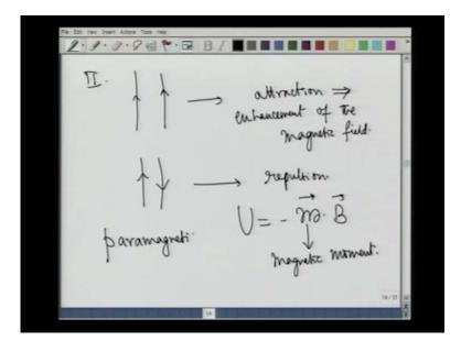
So, the analogy, analogous to dielectric response, but on the other hand, we said, that if the currents are already existing, so that is the scenario number 2. If the currents are already existing, so let me imagine, that there are 2 parallel wires, I am looking at a section of a large circuit, let us say, you can also look upon it as 2 magnetic moments, then these attract. So, here you see, they tend to enhance the magnetic field.
