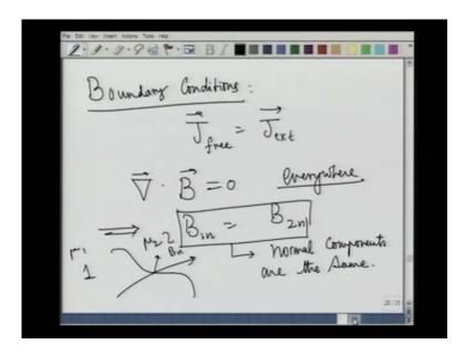
Obviously, I am now going to look at different media with different magnetic permeabilities, is that right, relative permeabilities. And I will ask, how should H change across the boundary and how should B change across the boundary?
