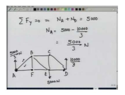
Once I know N D, then summation F Y is equal to 0, gives me N A plus N D is equal to 5000. And this gives me N A to be 5000 minus 10000 over 3, which gives me 5000 over 3 Newton. So, now if I look at this truss try to make it to scale. Now, I know there is a force acting here 10000 Newton over 3. There is a force acting here downwards 5000 Newton. There is a force acting upwards here 5000 over 3, and this is A B C D E and F.
