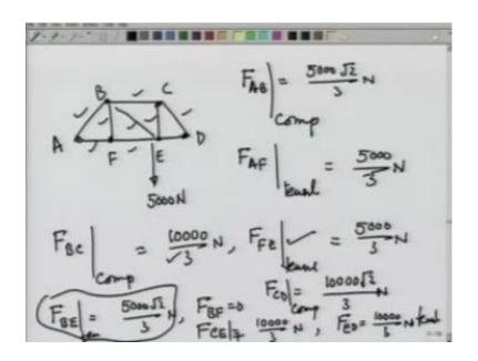
Earlier as we can see F B C was compressive 10000 over 3 Newton. So, we have learned two methods of analyzing forces in a truss.
