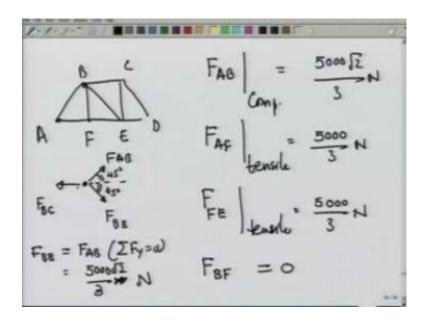
We have determined F A B and F A B was a compressive force compressive, and its magnitude was 5000 root 2 over 3 Newton. We have determined F A F, which is tensile, which is equal to 5000 over 3 Newton. We have determined F F E, which is also tensile and its magnitude is 5000 over 3 Newton. We have determined F B F to be 0. We are now rate and analyze point B.
