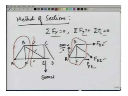
In which case, we cut a section through the truss. So, that maximum of 3 members are cut, and then I have 3 equations to solve namely summation F X equal to 0 summation F Y equal to 0 and summation tau A B out some point equal to 0 that give me those 3 forces. Let me illustrate, this method again by the same truss that we have solved. So, far A B C D E and F, and here is a load of 5000 Newton.
