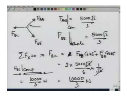
And F B C working this way, F A B is pushing the pin out. So, this is compressive is 5000 root 2 over 3F B E. We have just determined, but F B E pulls the pin N and therefore, why Newton third law pin pulls it out. This is tensile while its magnitude is 5000 root 2 over 3 and F B C from summation F X equal to 0 would come out to be 2 times the X component of F A B or F B is the same thing.
