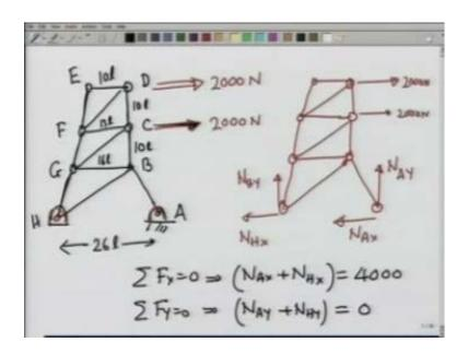
This is a truss like this where the lower point here is fixed. These are joined like this by rods, and this point is also joined by rods and this point is then fixed here at point A. So, this is a truss A B C D E F G and H notice that these likes H G, G F, and E F are slightly slanted B C and D C are vertical. This is 101 in length. So, is E D 101, this is 131 F C is 131 GB is 161, and this length is 261.
