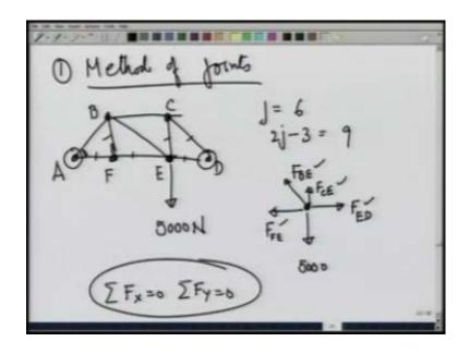
So, I will take a simple truss like this each angle being 45 degrees. These are the joints, you can see, there are 6 joints. So, j equals 6, 2 j minus 3 is 9, and there are 1 2 3 4 5 67 8 9 members. I am going name this A B C D E and F and apply a load of 5000 Newton at E. I want to calculate the force in each member of this truss. So, ideally if I start with this point, I would take point E.
