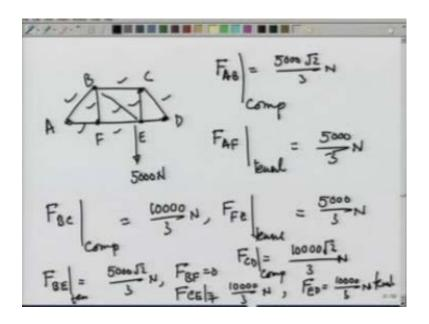
All the forces that we have calculated are A B C D E F when these truss is loaded with the 5000 Newton load at point E are F A B, which came out to be 5000 root 2 over 3 Newton and this was compressive. Then, F A F, which was tensile and it came out to be 5000 over 3 Newton. Then, F B C which came out to be compressive, and its value was 10000 over 3 Newton. Then, F F E which came out to be tensile again, and its value was 5000 over 3 Newton 1 2 B C,F E are done 4 1 2 3 4 members.
