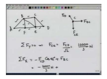
At this point we can also make a consistency check because at this point, if I have done my calculations correctly the X component must vanish automatically. That it does, we can see, because this is F C D with a negative sign cosine of 45 degrees plus F B C, F C D was calculated to be 10000 over 3 root 2. So, this comes out to be minus 10000 over 3 Newton plus F B C was calculated to be.
