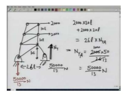
So, if I apply torque about point H. This is 10 10 l, this is also given to be 10 l. Then, by torque equation, I will get 2000 times 30 l plus 2000 times 20 l should be equal. This is N Y 26 l times N Y at A, and this gives me N Y A at point A equals 2000 times 50 divided by 26. That is100013 equals 50000 over 13 Newton in the direction shown.
