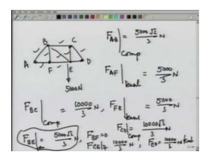
We had obtained F B E to be tensile of 5000 root 2 over 3 Newton.
