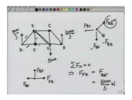
If, I make it again, I know the force here is 5000 over 3 force here is 10000, over 3 force here is 5000. I know the force in this member, and in this member. Now, if I go to point F A B C D E or point B. I have 2 all the 3, I have 1 force, which is known and therefore, I can calculate the other 2 forces. Let us go to point B, the pin at B is under equilibrium due to a force on A B, which is compressive.
