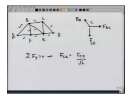
So, F B C was compressive and therefore, it will push point C. In this manner F C E is what we want to calculate and these are the 3 forces under which the system is in equilibrium right away. You can see that summation F Y equal to 0 would give me F C E to be equal to F C D over root 2.
