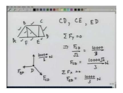
And we have already calculated F C D to be 10000 over 3 times root 2 Newton and therefore, we get this to be 10000 over 3 Newton.
