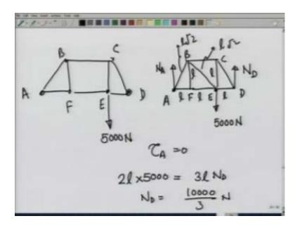
Let me make this again A B C D E, and F the force of 5000 Newton acting downwards. Let me take the entire truss as one unit, let the normal reaction at D be N D, let the normal reaction at A be N A. And there is a force acting downwards of 5000 Newton. I have not been careful in making this to scale. Let the length of this small state rods be l, so that this diagonal rods is l root 2, this length is also l root 2 and so on.
