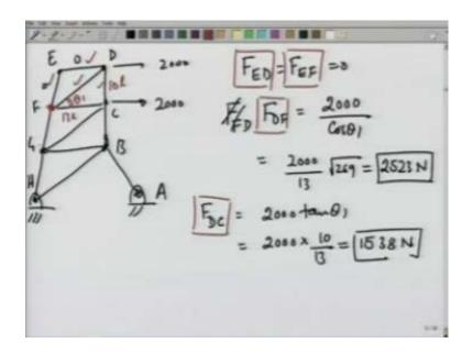
So, F D F equals 2000 over cosine of theta 1. Let me remind you, this is theta 1 this is 10 1, this is 13 1. So, which is equal to 2000 over 13 square root of 269. And F D C, D C comes out to be 2000 tangent of theta 1, which is 2000 times 10 over 13, which comes out to be 1538 Newton. Similarly, then F D F comes out to be 2523 Newton. So, we found the 4 forces F the box. Then, F E D, F E F, F D F, F D C, we found this, we found this we have found this, we have found this..
