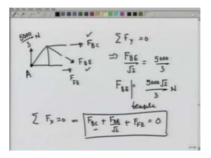
Now, using the equation summation F X equal to 0. I can also calculate F B C and let us do that.
