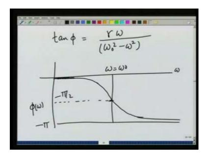
So, for very low frequencies if this is omega and I go to plot phi omega a very low frequencies the phase is almost the same as the applied force. So, the system is moving with the applied force then, at omega equal to omega 0 the phase lags behind the system lags behind by minus pi by 2 at omega equal to omega 0 this becomes 0. So, tangent phi is infinity.
