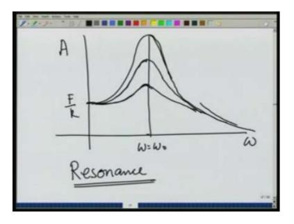
In between its behavior for light damping is something like this where the maximum occurs at omega equal to omega 0. If I increase gamma it will be something like this if I increase gamma further, will be something like this If you increase gamma the maximum shifts slightly to the left slightly to a value lower than omega 0. Of all practical purposes you can say that it is peaking at omega 0 and then far way it decays like this.
