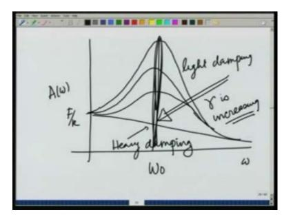
So, there is no maximum for heavy damping the curve just goes like this. Nonetheless the system does oscillate even in the case of heavy damping when, subjected to a an oscillating force. I can say that in this direction gamma is increasing. So, in light damping case I do have a resonance at this point omega 0 which really reflects that the maximum the amplitude becomes maximum at that point.
