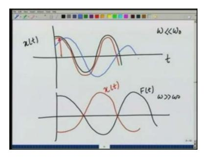
This is time xt let us, say this is omega much less than omega 0 a forces like this and in this case the displacement will also be following roughly the same graph I have not shown the amplitude correctly only the relative phases. On the other hand if, omega is much larger than omega 0 then, is the forces like this the displacement would be out of phase by pi this is xt black 1 is Ft.
