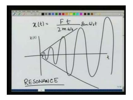
So, it will look something like this you see, this part goes up linearly this is the phenomena of resonance. So, when omega the applied frequency is exactly equal to the natural frequency the oscillations grow linearly with time and finally, the amplitude becomes very large. In fact, so large that the oscillator may break. I am doing this phenomena here for free oscillator.
