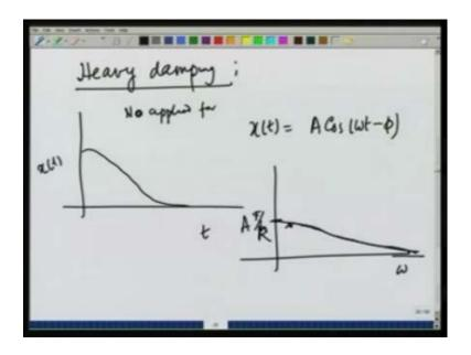
What happens? If I go to heavy damping. If you recollect the previous lecture we recall that in heavy damping without force no applied force the motion finally, came to a stop like this, but in this case no matter what the damping value is the motion will always be there oscillatory. Because, xt solution in steady state is some amplitude cosine of omega t minus phi.
