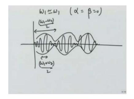
You will see that the solution would be of this form. So, the amplitude would be varying with time and the frequency of oscillation will be roughly equal to omega1 plus omega2 over 2 and this frequency of change of amplitude would be omega1 minus omega2 over 2. I would like you to do this exercise yourself by using by adding the 2 solutions. So, this is like the phenomena of beats.
