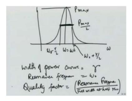
This is known as the width of power absorption curve. So, width of power curve is gamma resonance frequency is omega0. You see, right away that the quality factor is also related to the resonance frequency and the full width at half maximum. This is another way of looking quality factor q that we are introduced in the previous lecture. So, far we have looked at steady state solution.
