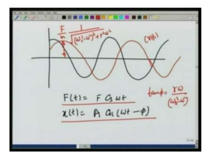
But if I will just look at the Phasor relationship is going to lag behind by this angle phi. If we translate this into the graph for displacement verses time The applied force is of the form cosine omega t Ft is of the form F cosine of omega t. whereas, xt is of the form some amplitude cosine of omega t minus phi.
