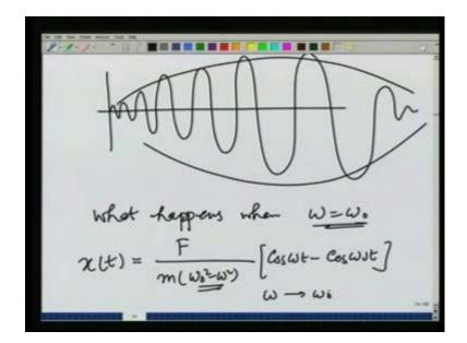
So, what would be very interesting question to ask now, is what happens? When, omega equals omega 0 recall, that the solution is xt equals F over m omega 0 square minus omega square cosine of omega t minus cosine of omega 0 t I cannot substitute omega equals omega 0 directly here. Because, when I divide it I assume omega and omega naught were not equal. So, I take the limit omega going to omega 0. So, let me take omega to be slightly smaller than omega naught and substitute it here.
