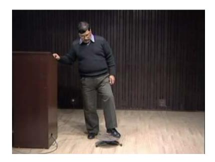
As the first example I take this platform which can be freely rotating. So, if I stand on it start rotating I will have an angular momentum about the axis. I will show you first the effect of how changing the moment of inertia changes my angular speed in order, that the angular momentum remains constant.
