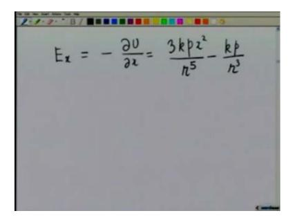
So, the expression for the electric field x component that I get is going to be x which I took to be the partial derivative of U with respect to x comes out to be 3 k p x square divided by r raise to 5 minus k p over r cubed.
