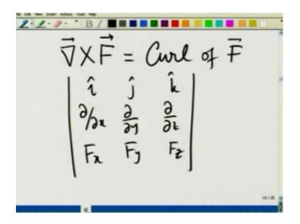
These are all components of a vector form by this which is known as curl of F and you can see this I j k this is by definition F x F y F z determinant, this gives me all three components that I wrote in the previous slide.
