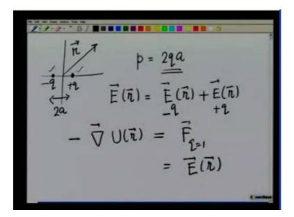
So, I am going to consider a dipole sitting at the origin with charge with minus q on negative y x axis and charge plus q on the positive side of the x axis with the distance between them being 2 a.
