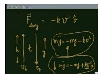
The example I take is that of F drag being proportional to v square. And obviously, it is in direction opposite to its velocity. And I want to find, if I throw a particle up with some initial speed, v initial, how long does it take to reach up? What is the height it can go up to? And what is the speed when it comes down? v final.
