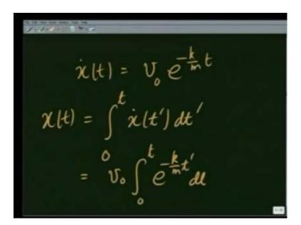
x dot t is given to be v 0 e raise to minus k over m t. So, the distance travelled in time t, is going to be integral 0 to t x dot, t prime, dt prime which is equal to v 0 integral 0 to t, e raise to minus k over m t prime, dt prime.
