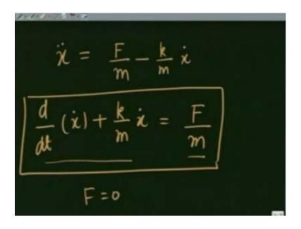
If I rewrite the equation will come out in the form of x double dot is equal to F over m, minus k over m x dot, or d over dt of x dot, plus k over m of x dot is equal to F over m. Notice, I have already solved this problem for F equals 0, that was 1 dimensional motion without any force. In such situations, where I have 1 part like this and another part like this, I can write my solution as the previously obtained solution with F equals 0, which was nothing but C e raise to, minus k over m t.
