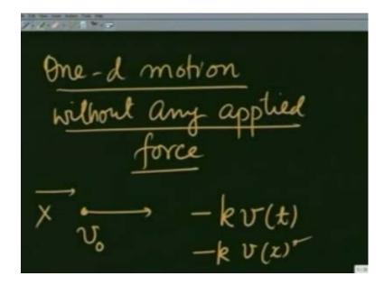
The first example I am going to take is going to be 1 dimensional motion without any applied force. There is no applied force, but drag is there. Therefore, initially I have to throw the particle with some initial speed v 0, and as it moves along it experiences a force which is minus kv, v is changing with time or I can also write v is changing with the distance. Let this direction be x direction that is I have written x here.
