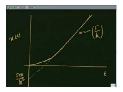
T xt initially it is going as t square and finally, it goes as a straight line. a straight line with slope F over k. which is nothing but the terminal speed and which cuts the y axis somewhere here, which is nothing but Fm over k square. So, this is how the particle is going to cover the distance with time. This is a problem where we applied a constant force. So, the most familiar problem in everyday life of this is a ball being thrown up with say some initial speed v 0.
