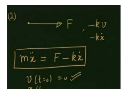
Next let us consider a particle still moving in 1 dimension, but applied on it is a constant force. So, I have a particle, I apply a constant force F again an x direction, and let there be a drag force minus kv or minus k x dot. And I want to solve how, I want see how this particle moves. The equation of motion is going to because m x double dot is equal to F minus k x dot.
