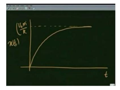
If I plot xt as a function of time. Initially obviously, distance travelled is 0, and slowly it moves up and goes like this, distance is being v 0 m over k.
