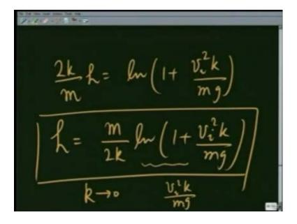
Or 2 k over m h, equals log of 1, plus vi square k upon mg, or the height it went up to is equal to m over 2 k log of 1, plus vi square k upon mg, this is the height at which it stops. Again, I will go back to limit of k going to 0 and see if my answer is correct. When the
