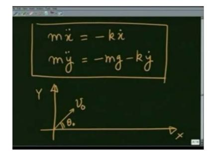
mx double dot is equal to minus k x dot because there is no horizontal applied force. And in the y direction, I am going to have m y double dot is equal to minus mg minus k y dot. These are my two equation of motion. When I am solving for a particle which is being thrown at an angle theta 0 with initial speed v 0, this I am taking to be positive y direction, this to be x direction. These two I have solved separately when I was solving the 1 d problem so, that I know the solution.
