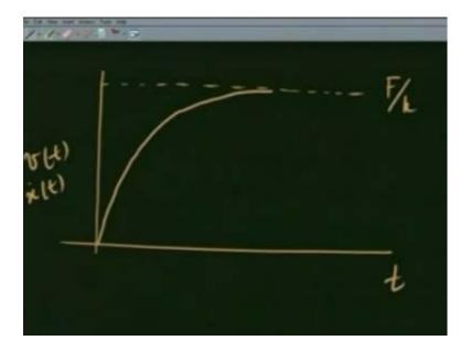
If I plot this speed I am going to get vt or x dot t same thing verses t, the final speed is F over k and the speed slowly builds up. How about the distance travelled? Well for that, I again integrate it.
