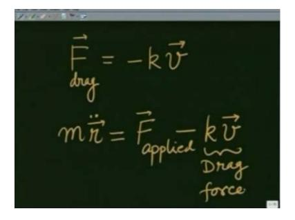
The simplest one as I said earlier is the force which is proportional to v, and I am going to write this as F equals minus kv. And I am going to call it drag force, k is the coefficient of drag, minus sign again denotes that, the force is opposite to the motion.
