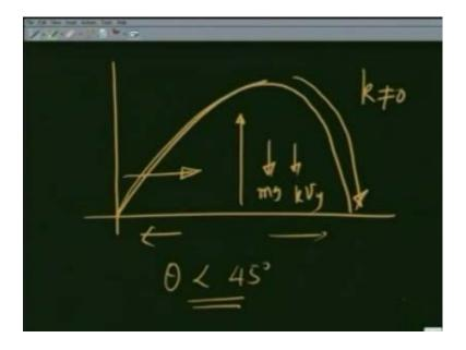
Because you saw that the height is not affected so much by introducing of k as the range. So, what I want to do is give slightly more of x component to the velocity, if I want to fire the projectile further and further. The other way to look at the same problem is that, when the particle is moving is up, it spends more time because it is being pull down by mg, it is also being pull down by kV y spends more time in going the same height then, when it is coming down.
