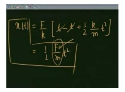
And expanding it further I get xt equals F over k, t minus t plus 1 half, k over m, t square, which is nothing but you are familiar 1 half F over m, t square which is the correct answer in the limit of k going to 0. That is I am taking particle and applying a constant force F, its acceleration is F over m, and there it moves distance 1 half F over m, t square in time t. Let us try to plot this and see how it goes.
