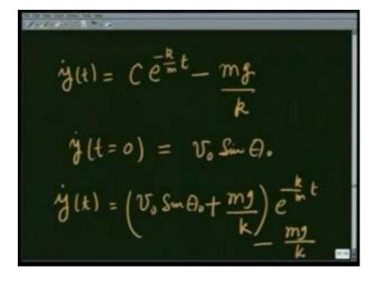
And therefore, y dot as a function of t is going to look like C e raise to minus k over m t, minus mg over k. And C is determined by the initial condition which is that y dot at t is equal to 0, is equal to v 0 sin of theta 0. And therefore, I have y dot of t is equal to v 0 sin of theta 0, plus mg over k, e raise to minus k over m, t minus mg over k.
