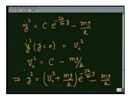
So, I have y dot square equals some constant e raise to minus 2 k over m y, minus mg over k, and I know the initial velocity y dot square, when y is 0 is equal to v initial square. And therefore, v initial square is going to be equal to C, minus mg over k and that gives me y dot square is equal to vi square, plus mg over k, e raise to minus 2 k upon m y, minus mg over k.
