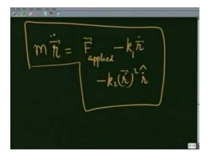
Because now you have m r double dot is equal to F applied, minus k r dot k 1 r dot, minus k two r dot square r dot vector. And these are not easy to solve. In most of the cases, you have to apply numerical methods to get the final solution. However, there are
