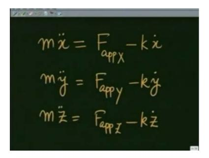
If I write these in component form I get mx double dot equals F applied x component, minus kx dot, my double dot equals F applied y component, minus ky dot and similarly, mz double dot equals F applied z, minus kz double dot. This is the simplest of drag forces and in the next few examples, we are going to see how to incorporate this in the motion.
