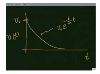
So, initially the particle started moving with some speed v 0, I am plotting vt verses t, and as time passed, velocity decreases exponentially. This curve is v 0 e raise to minus k over m t. How about the distance travelled by the particle? That is also easy to calculate once I know the velocity.
