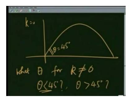
If k is equal to 0, the maximum range which is attained is when theta is equal to 45 degrees. What theta for k not equal to 0? Is theta less than 45 degrees? Is theta more than
