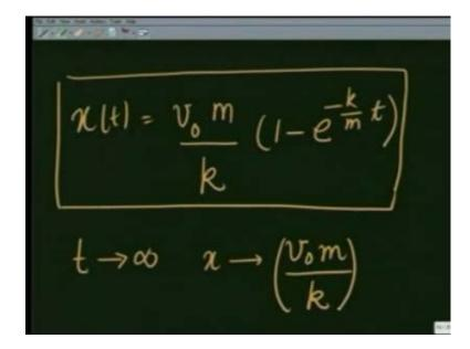
After integration I get xt is equal to v 0 m over k 1, minus e raise to minus k over m t. So, I have also calculated, how much is the distance travelled in time t. As t goes to infinity, x goes to v 0 m over k. So, that is the distance that the particle will finally, travel and stop after this. Let us see how does the plot of this look.
