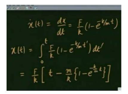
So, I have x dot t, equals dx dt is equal to F over k 1, minus e raise to minus k over m t. So, x at t is again going to be 0 to t, F over k 1, minus e raise to minus k over m t prime, dt prime integrating, I get F over k, t minus m over k, 1 minus e raise to minus k over m t. So, this is going to be the distance travelled by the particle. Now, that we have gotten
