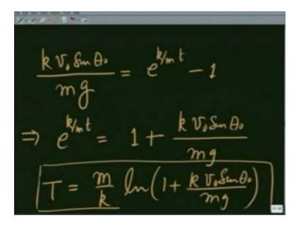
Or k v 0 sin theta 0 over mg is equal to e raise to k over m t minus 1, which implies e raise to k over m t is equal to 1 plus k v 0 sin theta 0 over mg or time T, when its velocity becomes 0 or reaches highest point is equal to m over k log of 1 plus k v 0 sin theta 0 over mg. Let me again ask and check my answer. Is this correct in the limit of k going to 0? Sure it is.
