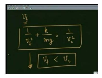
The velocity v final then, the relationship between v final and v initial square is going to be 1 over v final square, plus k over mg is equal to 1 over v initial square. The word of caution though, when considering the motion of part of the coming down you should take proper account of the force of friction.
