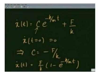
And therefore, my general solution for x dot is going to be x dot of t is equal to C e raise to minus k over m t, plus F over k. This constant C is again determined by initial
