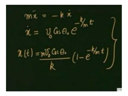
mx double dot equals minus k x dot gives me x dot, is equal to v initial, which in this case happens to be v 0, cosine of theta 0 e raise to minus k over m t. And also x as a function of time comes out to be v 0 cosine theta 0 m, over k, 1 minus e raise to minus k over m t. This is the motion in x direction, and this is related, this is going on concurrently with motion in y direction, for which I have.
