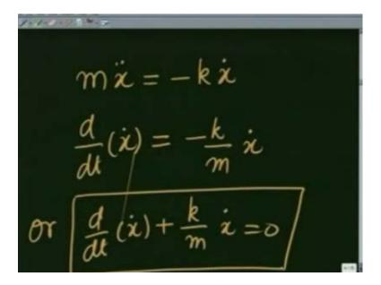
The equation of motion for this is going to be mx double dot equals, minus kx dot. In more familiar terms, it is going to be d over dt of x dot which is nothing but x double dot
