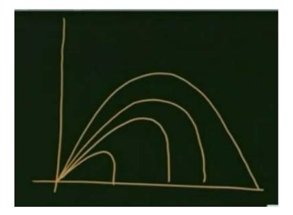
If I do that for different case, and a fix v naught and sin theta naught, I find that for k equal to 0 it is a perfect parabola. However, as k is introduced that means, drag force comes into play, its height and range both start changing and all have got some numbers here, which I will show you how for different parameters it changes. As an example of how the trajectories are affected for different values of that coefficient or by this drag.
