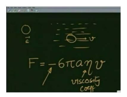
When a spherical body of radius a, moves through a gas or fluid at speed v, it is moving with speed v then, there is a force on a due to viscosity which is F equals minus six pi a eta v. This minus sign denotes that, the force is opposite to its direction of motion, eta is the viscosity coefficient. This is 1 example of the drag force that anybody moving through a fluid or gas experiences. Of course, this is the lowest order force.
