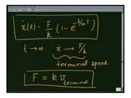
So, I have x dot t equals F over k 1, minus e raise to minus k over m t. We notice as t goes to infinity, that is after a long time I have applied the force x dot goes to F over k. This is nothing but the terminal speed, at this speed the applied force F becomes equal to k times v terminal. The two forces balance and therefore, the particle moves with a constant speed of v terminal.
