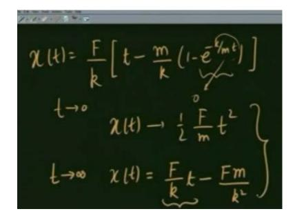
So, xt was F over k, t minus m over k, 1 minus e raise to minus k over m t, again in the limit of very small t. Basically making this term very small, we just saw that xt goes as 1 half F over m, t square.
