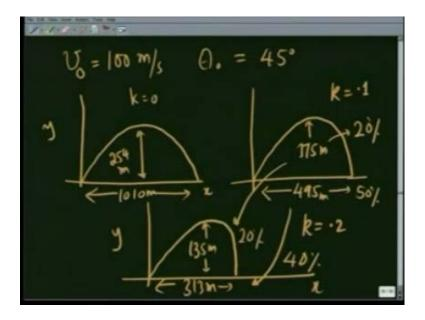
I have taken a sample problem of a particle being thrown in the speed of 100 meters per second at an angle theta 0 equal to 45 degrees, and I will plot for three different case, the
