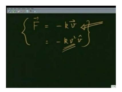
I have considered the simplest possible form where F is proportional to the velocity itself, and another form where F is proportional to the velocity square. This is encountered when velocities are small and suffices in most of the cases.
