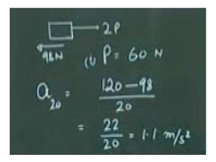
So, let us see what happens when I apply a force of 2 P here, and this is 98 Newton's. In case of P is equal to 60 Newton's, which was my case. The acceleration of the upper
