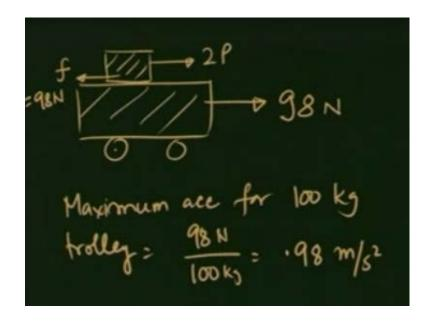
This fellow is moving this way, maximum force it can have in this direction 98 Newton's, this is has a force 2 P, and this has a force f maximum 98 Newton's. So, the maximum acceleration for 100 kg trolley is equal to 98 Newton's over 100 kg, which is 0.98 meters per second square. If the acceleration of the top mass 20 kg is happens to be larger than this then, there will be sliding, if it is less then, there will be no sliding.
