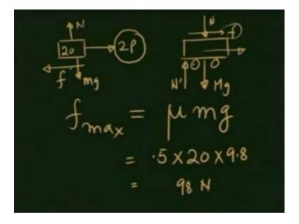
A free body diagram for the 20 kg mass is 2 P this way, friction this way, and for the trolley is friction this way. So, the trolley would move in this direction, and accelerate in this direction due to this frictional force. The 20 kilogram mass will also move in this direction because of 2 P and the force.
