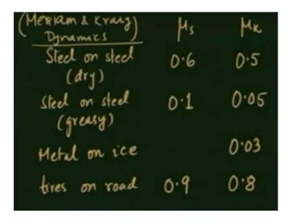
So, this is we will take steel, on steel dry surface. We will take steel on steel, greasy surface, and we will also take metal on ice, and tires on road mu, static for steel on steel is about 0.6 when they are both dry. Steel on steel on greasy is 0.1, you can see why we grease steel, it reduces a friction value quite a lot. Metal on ice, static is not known because slips passed were lot and tire on road is 0.9.
