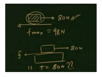
Maximum frictional force, this is 80 Newton's and f max is 98 Newton's. So, the friction will adjust itself just to 80 Newton's so that, this fellow, this mass does not slip. And therefore, you can conclude that, in this case, this is going to be 80 Newton's and there is going to be just sufficient force f so that, this does not slip. Is f equal to 80 Newton's? The answer is obviously no. You can see it in two ways.
