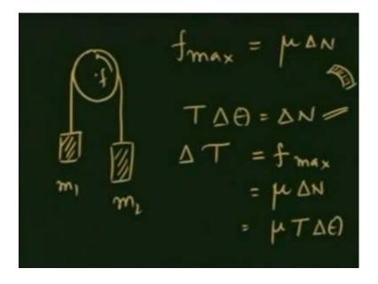
Let us now take the extreme case of when mass m 2 just balances mass m 1, this is the friction. So, that in that case friction is going to be maximum, and that is going to be equal to mu delta N on that small piece. So, I have equation from a layer T delta theta equals delta N, and delta T equals f max which is mu delta N which in turn from this equation is equal to mu T delta theta. So, I have a relationship between the tension change in it with respect to a change in theta.
