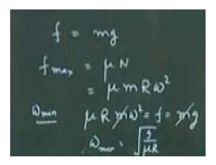
And the other equation gives me f equals mg. Remember f max is mu N so, that is going to be mu m R omega square. For the minimum omega. I should be applying the
