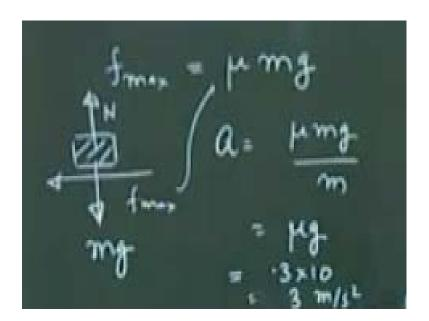
So, let us see what is the maximum friction f max is going to be mu mass of the box times g because for this box which is not moving in vertical direction, N is same as mg. So, f max is given by this formula. So, maximum deceleration a is going to be mu mg divided by m which is equal to mu g, which in our case if I take g to be approximately 10
