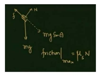
This body has weight mg, N, friction F, and mg this component of mg is pulling it down, which is mg sin theta. As I increase theta, mg sin theta goes up so, the body is being pulled down by larger and larger force. When it surpasses, the maximum possible frictional force it will starts sliding down. Let us see, what is maximum possible frictional force. Friction maximum as I told you earlier, is equal to mu s times N. N as we saw in the earlier.
