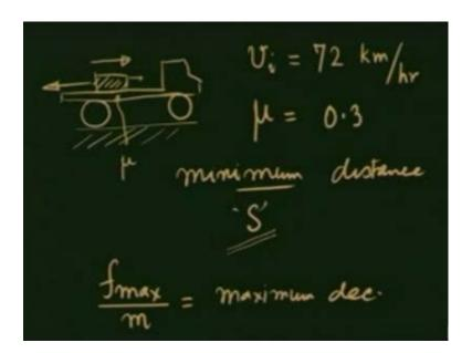
The first problem is if I have a truck moving at a certain speed and suppose there is a box here, the truck suddenly breaks, you know from experience if the truck breaks the crate or the box is going to move this way. If I am given the coefficient of friction here, that is
