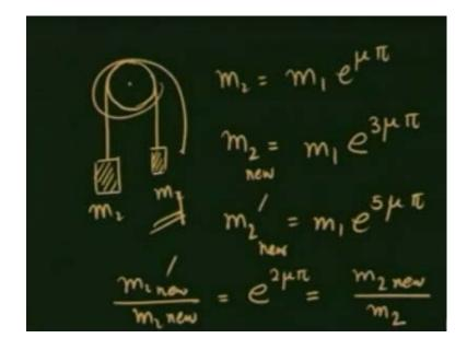
You take a pen and put a small object, may be a pen or a key on one side, and a large object on the other side of a string and try to balance it. As we said earlier suppose, this mass is heavier, m 2 would be in this case be equal to m 1 e raise to mu pi.
