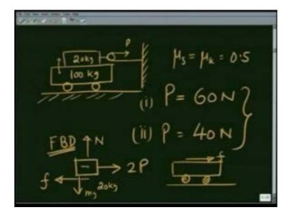
As a second example, I take a crate or a trolley which can move on its wheel without friction. This is taken to be 100 kilograms, on top of it I put a box of 20 kilograms and pull it with a pulley here, pull it by a force P other side of the string attached to the wall. The coefficient of friction whether static or dynamic, let us take it to be the same, between these two masses is given to be mu s almost the same as mu k is equal to 0.5.
