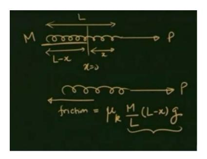
Partially from x equal to 0, the chain is like this, is being pulled by force P, let this distance be x, let the total length of the chain be L, this then it is going to be L minus x, let the mass of the chain be M. And I want to know when the chain has come out to fully form rough, what is this P?
