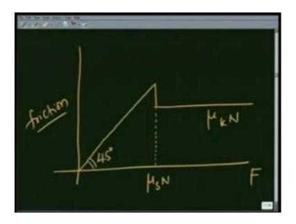
Let me redraw it for clarity so as I take a body, apply a force, the frictional force increases in proportion to the applied force, this as I said earlier is 45 degrees. And then, when it reaches the maximum mu s N, the body will start moving and the friction force drops slightly, this value being mu k N. To give you a feel for what mu s and mu k are, let me give their values in the next slide. For some materials, the value varies from material to material.
