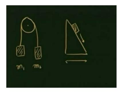
Two examples that we took were one acquits machine where I had two masses moving around a pulley m 1 and m 2. The other example that we took was a mass sliding down a wedge like this, and the wedge could also move horizontally. In these examples we ignored a ubiquitous force, that is encountered everyday in our lives, and that is the frictional force. This lecture is going to be about, how do we take into account the frictional forces, and how does it affect the motion of a particle.
