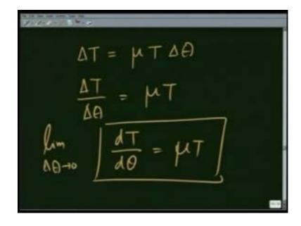
That gives me delta T equals mu T delta theta, or delta T over delta theta equals mu T limit delta theta going to 0, it gives me dT over d theta equals mu T. This equation is quite easy to solve, and you have being doing it in many different places, the solution for this comes out to be.
