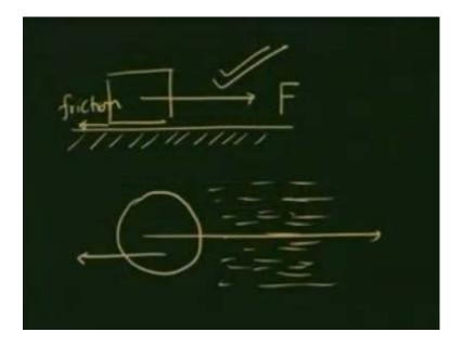
There are, when the body moves we see that its motion is usually resisted by the surface on which it is moving. So, if I apply a force F this way, there is the surface applies a force called frictional force that opposes this motion. Even if the body is not moving frictional force has a tendency to oppose a tendency to move.
