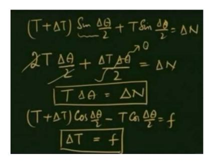
Let us then try these equations again I have T plus delta T, sin delta theta over 2, plus T sin delta theta over 2 equals delta N, which can be approximated for a small delta theta as 2 T delta theta over 2. I replace this whole thing by delta theta by 2, plus delta T delta theta over 2 equals delta N.
