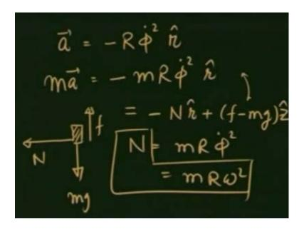
A is equal to minus R phi dot square r, ma therefore, is minus mR phi dot square r. How about the forces on the mass? There is a force in negative radial direction N, there is mg and there is friction. So, this should be equal to N in negative r direction, plus f minus mg in z direction. Equating the two sides, we get N is equal to mR phi dot square which is nothing but mR omega square.
