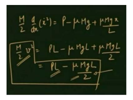
So, by integration I get I am integrating the equation M by 2, d over dx x dot square equals P, minus mu Mg, plus mu Mg x over L, by integration I get M over 2 v square
