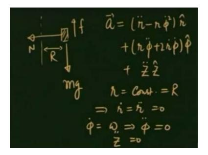
This is at a distance equal to radius of the cylinder from the center is being pulled down by weight mg, there is force N on it, and there is frictional force f on it. Its acceleration in cylindrical coordinates is going to be r double dot, minus r phi dot square r, plus r phi double dot, plus 2 r dot in phi dot in phi direction, plus z double dot z in z direction.
