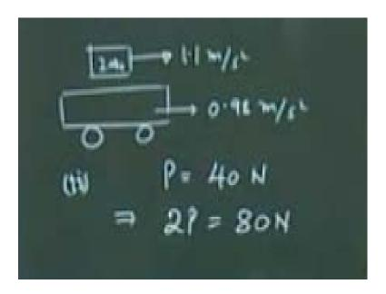
And therefore, in this case the two masses the 20 kg mass and the trolley are going to have acceleration. This is going to move with 1.1 meters per seconds square, and this is going to move to 0.98 meters per second square, and they are going to slip on each other. Let us see, the other case when P is equal to 40 Newton's which implies the 2 P is going to be 80 Newton's, and in this case 2 P happens to be less than the maximum force.
