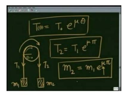
T equals some T 0 e raise to mu theta, where this T is being measured as a function of theta, T 0 is at T theta equals 0. So, let me just again make a picture and show you that this was mass m 1, this was mass m 2, T 1, T 2, theta is increasing this way, T is increasing this way, and if I take this to be theta equals 0, as theta increases theta also increases.
