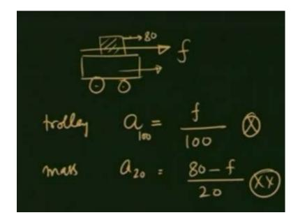
The answer is no because you see the trolley has only one horizontal force acting on it, that is the frictional force, there is nothing to stop it. So, the moment there is friction, this trolley is anyway going to move, if it moves and there is no slipping between the upper mass and the lower mass then, this mass is also going to move and both move in the same acceleration.
