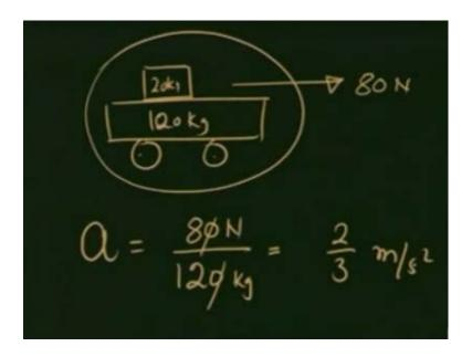
First if I consider the trolley and the mass sorry, 100 kg, together then, on this entire system there is a net force 80 Newton's, there is no relative acceleration, they are moving together. And therefore, their acceleration together is going to be 80 divided by 120 which is Newton's kg, which is going to be two-thirds meters per second square. But what about the frictional force in between? The question we started with is, is it 80 Newton's?
