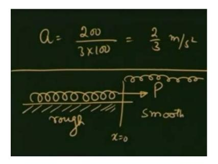
And that gives me the acceleration a, 200 over 3 times of 100 equals two-thirds meters per second square. So, you see how friction changes the acceleration, and how it affects the motion between two bodies that can apply frictional force on each other.
