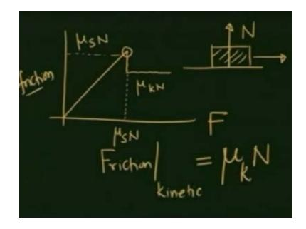
Of course, once the body starts moving the frictional forces slightly less. So, that I write as friction kinetic, and it is given by mu k, the normal reaction.
