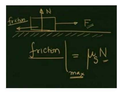
So, for example if I take a mass sitting on a surface and I try to pull it by a force F, it will, its tendency to move would be opposed by this frictional force. It is observed experimentally that the maximum frictional force that a surface can apply on a given mass is given by mu, where mu is a constant times N and I will put a subscript s here, to indicate that this is static friction. Friction is slightly different when the body starts moving, and we will be discussing that.
