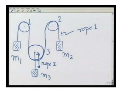
So, what we are going to do is take two fix pulleys, they are fixed at some height, pass a string of fixed length over them and the string turns around with the help of this third pulley.
