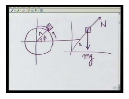
Since, the motion is circular because before leaving the drum the block is moving in a circular path here. I am going to use planar polar coordinates, taking this angle as phi increasing this way, and r obviously, is the radius.
