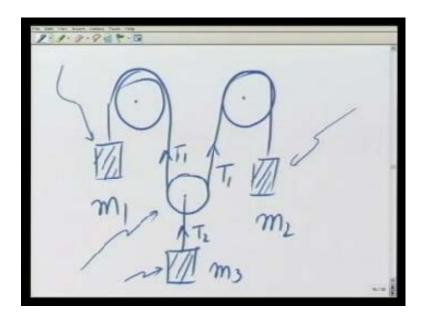
This is my pulley, mass m 1, here is a pulley, here is the other pulley, mass m 2, m 1, m 3. Here the tension works this way T 1, T 2, these are the forces of constraint. Again I am assuming T 1 and T 2 to be the same because I will be considering for simplicity massless and frictionless pulleys and assume that all the ropes are massless.
