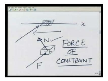
That is a mass or a bead moving on a straight wire as I set in x direction let us say, through this example, I would like to introduce terminologies that are going to be in use, when we talked about, when we talk about constrained motion.
