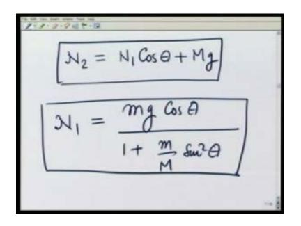
But that N 2 is equal to N 1 cosine of theta plus Mg, which tells you that N 2 balances the all the vertical forces acting on the wedge. The other equations when substituted for, would give you a result for N 1. I leave the solution and substitution and all those things for you, give me the final answer which gives you N 1 is equal to mg cosine of theta divided by 1 plus m over M sin square theta.
