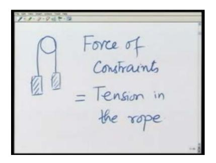
See what is causing the constraint, the constraint is caused by this rope that forces the two masses to move together. What is the force of constraint here? The force of constraint that really makes the masses to move together is nothing but the tension in the rope. So, tension in the rope is the one that keeps these masses together. next if I go to make the free body diagram for the two masses.
