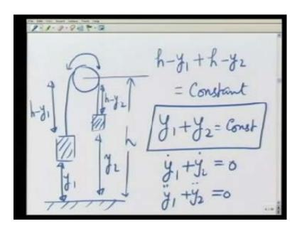
And that is where this picture comes in handing. We call again the constraint that, the two masses move together is provided by the fact that, the rope is of fixed length. And I can express this mathematically as this part which is h minus y 1, plus this part which is h minus y 2, plus this part is of constant length.
