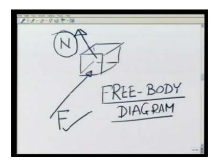
I am making it slightly bigger now is just to produce a force N or a force of constraint. If you look at this body, I have replaced the wire by this force of constraint, this is known as the free body diagram of it is a particle or a body under motion.
