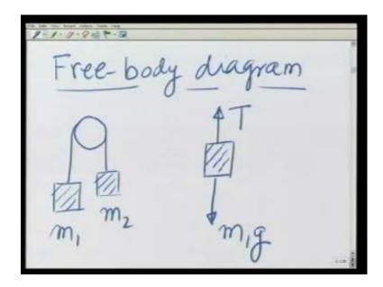
Let me remind you again, what a free body diagram is. A free body diagram is where I replace the agency causing the constraint by the force of constraint there it applies.
