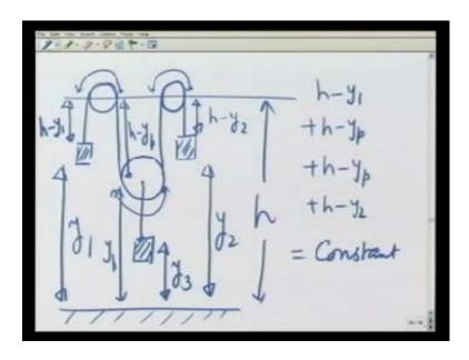
Let us do that, and for that again we go back to our diagram where I will now take the constraints into account that, the lengths of these ropes, both the ropes are the same, are fixed. So, this is y 3, these were at height h from the ground, this is at y 2, this is at y 1.
