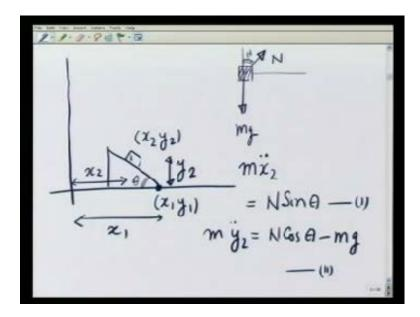
And for that what I am going to do is, make the wedge here, this is the block. For convenience I will choose this point to represent the coordinates for the wedge. Let this be x 1 y 1. Notice since, I am putting this constraint that, the wedge moves only in the horizontal direction, I am explicitly writing y 1 and later I am going to eliminate this using the constraint equation.
