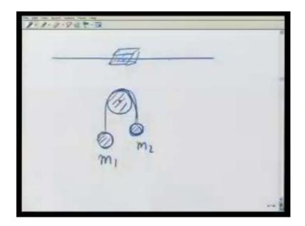
The constraint was caused by this wire or by other body itself, that is in this case this mass m 1 and 2 when they were connected by this rope this was providing the tension. But the presence of one mass restricted the motion of the other mass. And also when we solve these two simple problems that, you already knew the answers of, we also tried to develop stepwise strategies to solve motions of different bodies when they are moving under constraints. Let us try to right them.
