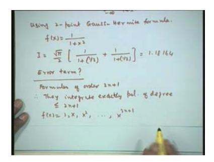
Now as I said these are formulas of order 2 n plus 1 therefore they integrate, they integrate exactly polynomials of degree less than or equal to 2 n plus 1 that means if I take f(x) is equal to 1, x, x square, so on x to the power 2 n plus 1, then these formulas will integrate exactly.
