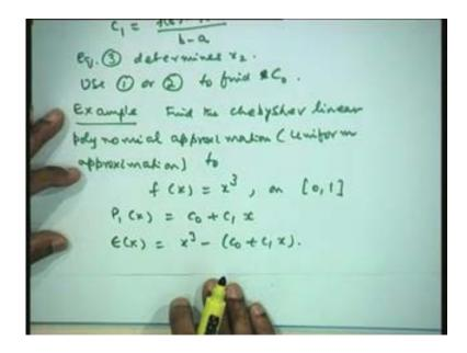
Now as we have done just now, let us take the required approximation  $P_1(x)$  is equal to  $c_0$  plus  $c_1x$  and define our error as epsilon(x) is equal to x cubed minus  $c_0$  plus  $c_1$  x. Now I need to choose 3 points in the interval 0 to 1 including the end points.
