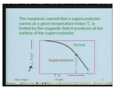
Same thing I have shown here here rather than the magnetic field produced here the current density critical current density c stands for critical and that is the critical value at this temperature that if the current flows from more than that it becomes a normal conductor and current remains less than that it is a superconductor.
