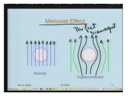
Now this is what I have talked about is the superconducting state of a material does not allow the magnetic lines of force to pass through it. However, there is always surface that is small thickness of the material where does it pass through this small surface is called skin and skin could range few times of angstroms upto 100 angstrom it could be. So around that thickness field can pass through but inside field magnetic field is not passing this is what shown here.
