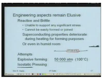
Now why we are not knowing all this having the material Yttrium Barium Copper Oxide we are not able to exploit even we cannot use it even for small simple application what talk about the transmission (())(44:52) the long cables to carry the current over miles and miles of
