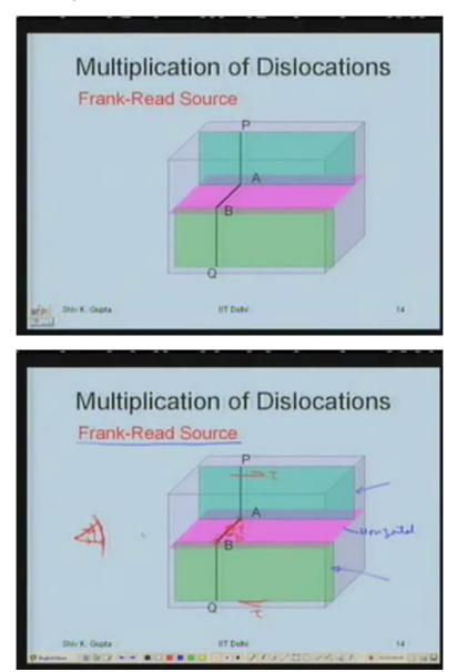
Wow, if that is the case that dislocations are responsible for causing plastic deformation in a material and once a dislocation gets out of the crystal is no more available to slip it can not cause any more further deformation so any dislocation which is present in the crystal gives me a step over equivalent to one burgers vector which is a permanent change in shape of the crystal only one burgers vector if I have let us say 100 dislocation in a crystal I'll get 100 burgers vector.
