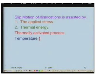
Slip Motion of dislocations is assisted by 1. The applied stress Thermal energy Thermally activated process Temperature † E = A exp(-
