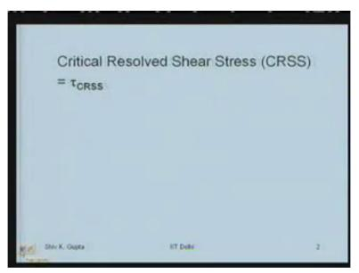
The critical resolved shear stress, is the minimum value of the stress at which plastic deformation occurs in the material and we saw that why we are talking about resolved shear stress mechanism of deformation by enlarge is a slip in most materials as most temperatures and then we saw that.
