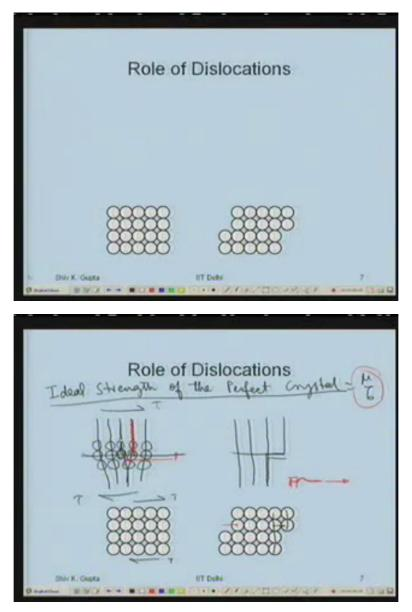
And this is how the slip or the deformation occurs in a material the semi fact can also be produced if I have and edge dislocation like this and I apply the shear stress in this manner so here also I am applying the shear stress in this manner and then it deform like this and you don't call that when I talked about slip motion of the dislocations this dislocation can go out ultimately and cause a permanent step like this.
