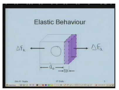
Now, while looking at the elastic behavior of materials, I consider again a very simple structure, simple cubic structure, unit cell, there is one atom sitting in the middle which is bonded on the 6 sides to other neighbors and I apply a small force in tension, this bonds will extend in this direction and let us say this unit cell has dimension is 0. And this extends in this direction by an amount let us say delta X, right?
