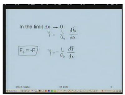
So I can write the Young's Modulus in the limit delta X standing to 0 as dFa divided Dx, if I use this I can write this as 1 upon a0 the minus sign dF by dx. F is the force between atoms and this is the applied force.
