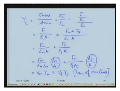
So let us write down the Young's modulus of the composite. Now we know the modulus of the matrix and the fiber are not the same, they are different materials. And strain is the same, the force taken by the matrix and the fiber is also not the same then and force I can then write as, force taken by the matrix plus the force taken by the fiber, this I can split.
