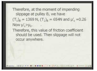
The most interesting of them all is mu s dash which is the coefficient of static friction at the pulley B which is point two six. So for the no slip condition at pulley A, it was point two one four. So the new coefficient of static friction is greater than the previous one. If we have this coefficient of friction, then there will be no slip condition at both pulley A as well as at pulley B. So this is the desired coefficient of friction which will eliminate the possibility of slip everywhere.
