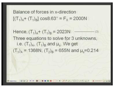
So we will take the components of the belt tensions in the horizontal direction. For example, on one side it will be T one A cosine of eight point six three degrees, on the other side also it will be T one B uh cosine of eight point six three degrees.
