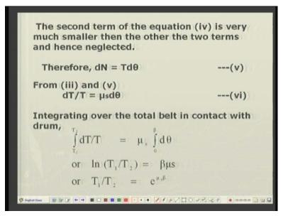
So it means, second term can be neglected in comparison to first and the third term and then the equation reduces to dN is equal to Td theta and combine the equation three and five. Five is over here and three equation is over here. So if you combine these two, then I have dt by T is equal to mu s times d theta, that is, the change in tension over the tension at that point is equal to mu s time the angle over which this change is taking place.
