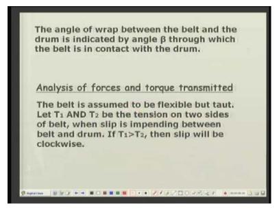
So let us see how we can analyze the forces and torque transmitted. Remember the tension on one side of the belt is T one, on the other side is T two and if the impending slip is to take place in the clockwise direction, then T one will be greater than T two, that is, the belt will be trying to slip like in this direction.
