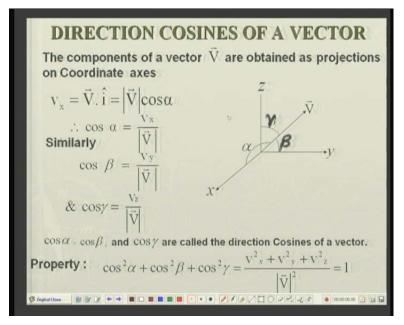
Similarly when you come to angle cosine beta, well then this is the angle between vector V and the y axis and this is the angle between vector V and the z axis. So each time you consider the unique plane containing the vector and the corresponding axis. So angle alpha is the angle between x axis and B, angle beta is the angle between y axis and V and angle gamma is the angle between V and z axis. Okay.
