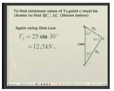
So both this cable tensions are easily obtained by a simple sine law of triangles and using the triangle law of addition of vectors. To find the minimum value of T2, it is a very easily understood graphically. Again, we have drawn the twenty five kilo Newton line, okay, and the direction of T1 is known to me. Of course, its magnitude is not known. Now, from point B, I will draw a line to represent T2, which will be the shortest distance between B and C. Okay.
