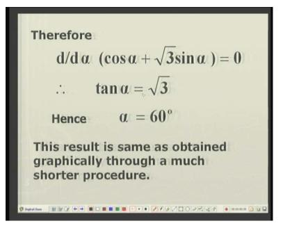
And this can be done by simple calculus, that is, the derivative of this expression should be equal to zero and when I take the derivative of this expression, I get tan alpha, which is equal to root three and hence alpha is equal to sixty degree. So again we come to the same conclusion, that when the second cable is inclined at sixty degrees to the vertical, the tension in that cable is minimized. Okay. (Refer Slide Time: 36:30 min)
