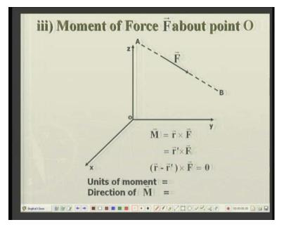
Let us now define a very important quantity associated with the force because this represents the turning action of the force. Force has two actions, one is push and pull and the other is the turning action. Now, suppose there is a force vector F, the line of action of this force is the line AB and the movement of this force about the given point O is defined like this: A movement M is equal to the cross product of the r and F. Okay.
