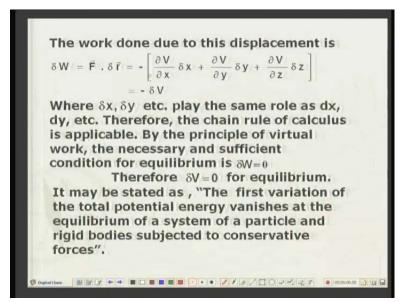
Then taking the dot product of the force with the virtual displacement, I will get the virtual work del W is equal to dot product of F with del r and if you carry out this product, then dV by dx into del x plus dV by dy plus del y plus dV by dz into d ah del z. That is exact nothing but minus of the del V, that is, the virtual where difference between the two positions of the potential energy.
