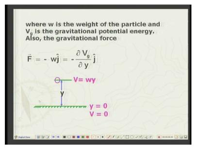
So I have illustrated this. Suppose there is a sphere or a ball of weight W, then at the ground level, that is y coordinate, the height coordinate is zero. So the potential energy is zero but when it has gone up, the potential energy will be w times y. If it goes down then it will be negative.
