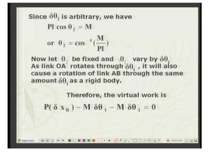
Once we substitute in to this equation and simplify, we will get theta two is equal to cosine inverse M over P l. So at equilibrium, the angle of the lower link to the vertical, that is, theta two
