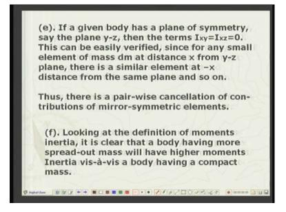
So, again, if the given body has a plane of symmetry, let us say, y z plane is a plane of a symmetry, then from the definition of the product of inertia terms, if I go back quickly to that definition, there is an element at a particular distance from that plane.
