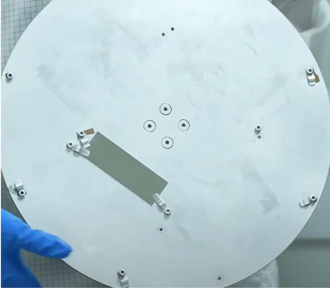
This is the aluminum which we deposited a while ago. and it is an ideal practice to again keep the chamber into vacuum condition or evacuated condition. So, I will again press cycle so that the chamber will go to lower atmospheric pressure and then finally we can stop the system as a whole.
