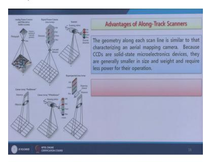
Further advantage is the geometry along each scanline is similar to that of characterizing an aerial mapping camera because CCDs are solid state, there is no moving part and they are generally smaller in size and and a weight and require less power for operation so another advantage is that they are lightweight and they are compact and the weight of a sensor onboard of a satellite is also less, it requires less power for operation.
