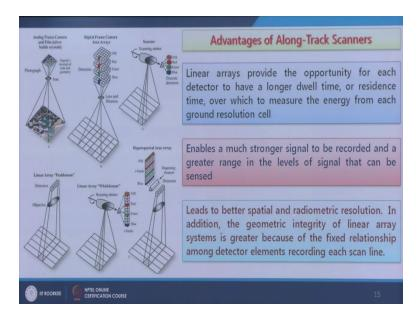
So the examples are shown here that the linear array or this the push broom, whisk broom, examples are shown and in hyperspectral area, then again the arrays are used so that along track scanning devices are used whereas in this one, this is rotating mirror so different channels are different pixels are gathered here whereas here the entire line or the swath is covered in 1 go so different way of collecting the data.
