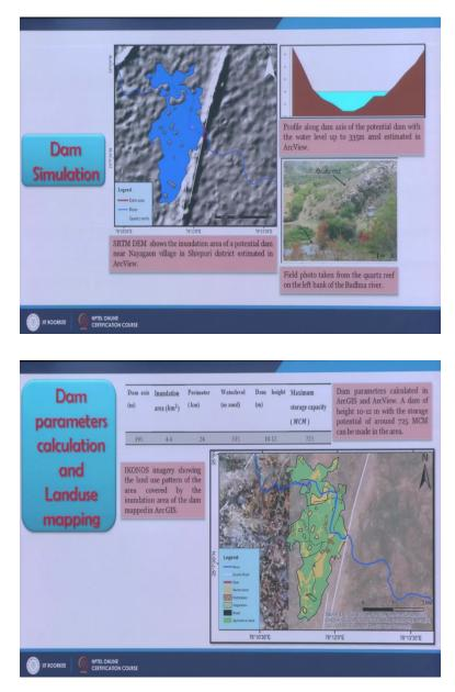
So, this is the quartz reef if a stream is going if it is blocked then a dam can be constructed and the simulation of dam has been done in GIS platform it shows that how much area if this much height of dam is created how much area will be inundated and so which land use will submerge that can also be estimated so that kind of work can be done starting from satellite image interpretations. So, thank you very much.
